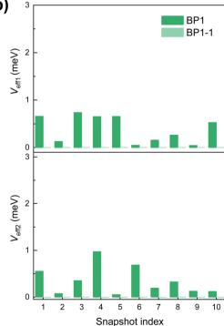
Fig. 4 Effective electronic couplings (absolute values) at 10 molecular dynamics snapshots of (a) BPc and (b) BP1. Absolute values of  $V_{\text{eff1}}$  and  $V_{\text{eff2}}$  of the superexchange process are calculated by eqn (3) and (4), respectively.
