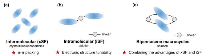
Fig. 1 Summary of characteristics in (a) intermolecular singlet fission (xSF) and (b) intramolecular singlet fission (iSF) and (c) the design strategy for bipentacene macrocycles.
