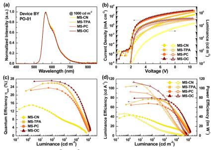
Fig. 8 (a) Normalized EL spectra at a luminance of  $10^3$  cd m<sup>-2</sup>; (b) current density-voltage-luminance (J-V-L) characteristics; (c) EQE vs. luminance; (d) luminance/power efficiency vs. luminance, for devices BY1, BY2, BY3, and BY4.
