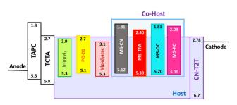
Fig. 3 Energy levels for MSs and other materials used in OLED devices.
