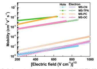
Fig. 5 Comparative field dependence mobility of MS-CN, MS-TPA, MS-PC, and MS-OC
