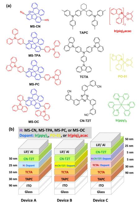
Fig. 6 (a) Schematics of the materials used in the OLEDs; (b) schematics of the fabricated OLEDs with different emitters.
