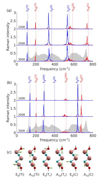
Fig. 3 (a and b) Raman spectra at different temperatures of Ti<sub>3</sub>C<sub>2</sub>O<sub>2</sub> and Ti<sub>3</sub>C<sub>2</sub>(OH)<sub>2</sub>, respectively. The blue lines represent the in-plane modes while the red ones represent the out-of-plane modes. The grey areas show the experimental results and the dashed vertical lines show the frequencies from phonon calculations using the MLFF. (c) Eigenmodes of Raman active modes
