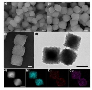
Fig. 1 Characterization of Mn-MIL-100@ZIF materials. (a) SEM image of Mn-MIL-100; (b) and (c) SEM images and (d) TEM image with the coresatellite architecture of Mn-MIL-100@ZIF; and (d) HADDF-STEM and corresponding element mapping images of the Mn-MIL-100@ZIF, illustrating the compositions of both MOFs in the Mn-MIL-100@ZIF heterostructure. Scale bars: 150 nm in (a)-(c), 200 nm in (d), and 170 nm in (e).
