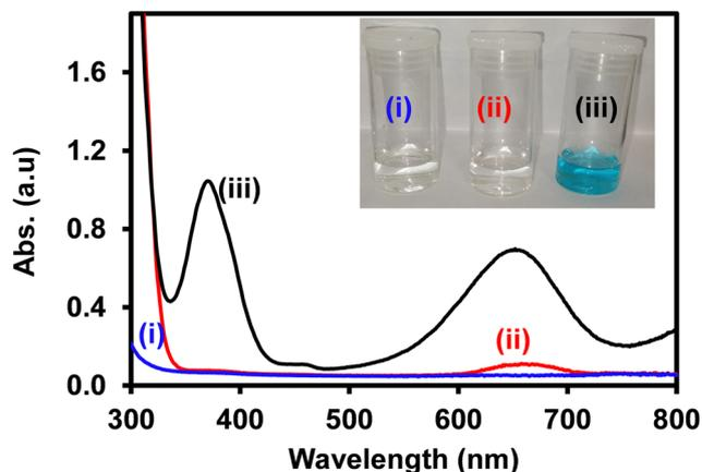
Fig. 2 UV-vis absorption spectra of (i) 0.20 M H<sub>2</sub>O<sub>2</sub> + ITO-SiO<sub>2</sub>-prS-PdNPs, (ii) 4.2 mM TMB + ITO-SiO<sub>2</sub>-prS-PdNPs and (iii) 0.20 M H<sub>2</sub>O<sub>2</sub> + 4.2 mM TMB + ITO-SiO<sub>2</sub>-prS-PdNPs (The inset photograph for the corresponding colour change of different reaction systems). All were measured in 0.20 M acetate buffer (pH 4.0).
