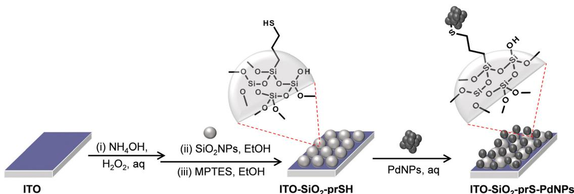
Scheme 1 Step-by-step fabrication of ITO-SiO<sub>2</sub>-prS-PdNPs as described in Section 2.5.
