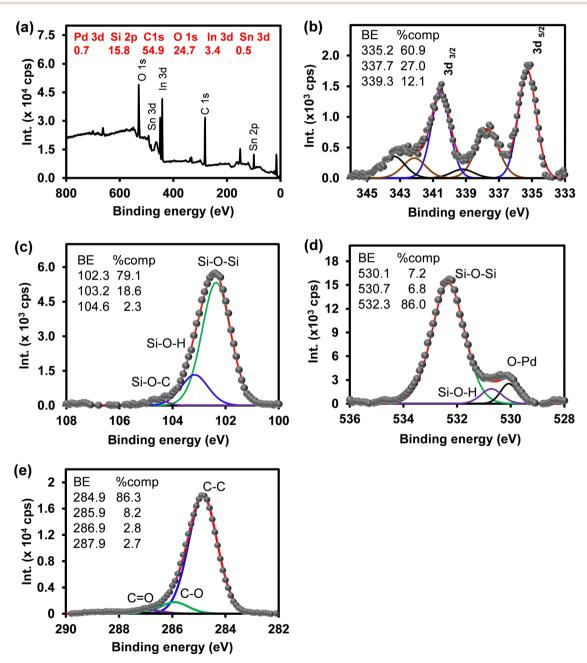
Fig. 1 (a) Survey spectrum and high-resolution spectra of (b) Pd 3d, (c) Si 2p, (d) O 1s, and (e) C 1s of ITO-SiO<sub>2</sub>-prS-PdNPs
