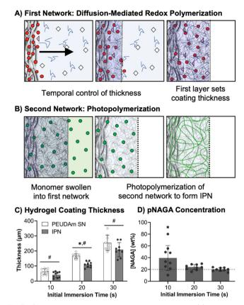
Fig. 3 Schematic of IPN hydrogel coating process. (A) Diffusionmediated redox initiated crosslinking of the PEUDAm first network sets the thickness of the hydrogel coating layer. (B) NAGA, bisAAm, and photoinitiators are then swollen into the first network and cured via photoinitiation. (C) Effect of immersion time on coating thickness of the first network and the second network at equilibrium state (n = 9). (D) Effect of immersion time on second network concentration (n = 9).
