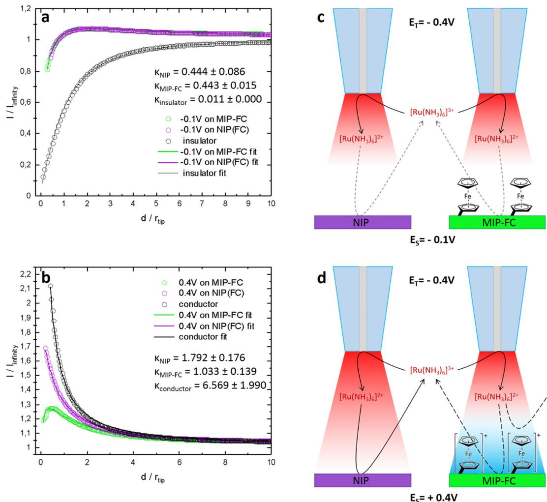
Fig. 7 SECM studies performed in feedback mode. Approach curves recorded on post-imprinting modified and non-imprinted macroporous film samples biased at (a)  $-0.1$  V and (b)  $0.4$  V vs.  $Ag_{pseudo}$ . Schemes showing post-imprinted and non-imprinted macroporous film behavior at (c)  $-0.1$  V and (d)  $+0.4$  V biased potential.  $E_s$ -potential applied to the sample electrode,  $E_T$ -potential applied over Pt microelectrode tip.
