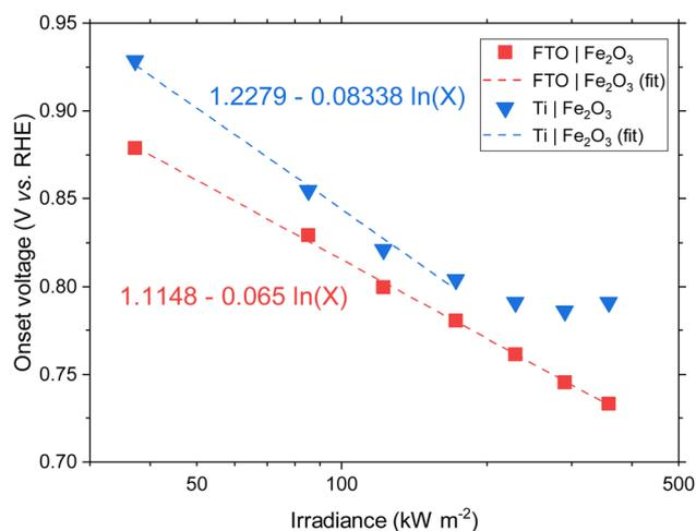
Fig. 5 Onset potential vs. irradiance for FTO|Fe<sub>2</sub>O<sub>3</sub> and Ti|Fe<sub>2</sub>O<sub>3</sub> and the linear fit. For Ti|Fe<sub>2</sub>O<sub>3</sub>, only the range 38–173 kW m<sup>-2</sup> are fitted.
