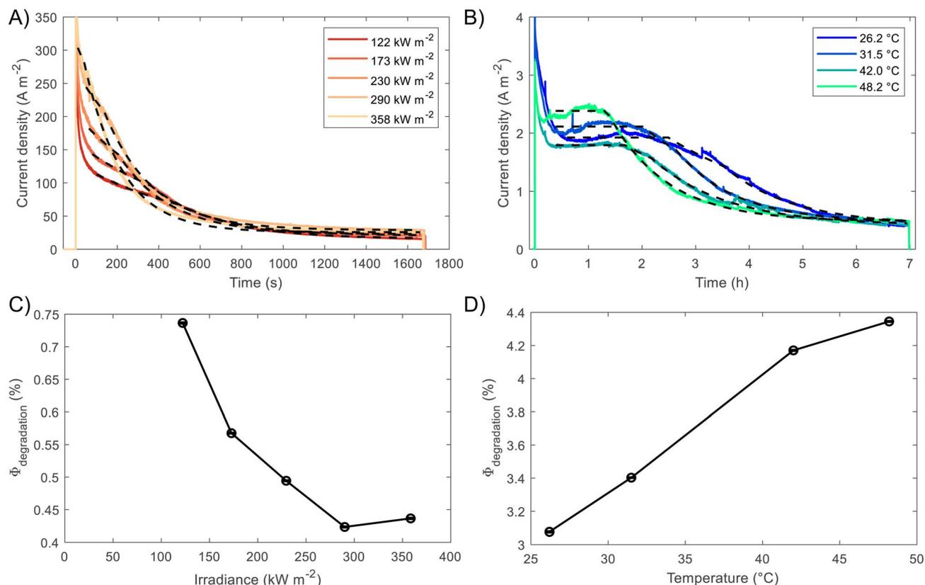
Fig. 7 Results of the model for prediction of BiVO<sub>4</sub> degradation. Experimental and predicted photocurrent densities at (A) different irradiances, 122–358 kW m<sup>-2</sup>, and (B) different temperatures 26–48 °C, under 1 sun = 1 kW m<sup>-2</sup>. (C) Estimated fraction of current towards degradation via dissolution of BiVO<sub>4</sub> as a function of (C) irradiance and (D) temperature.
