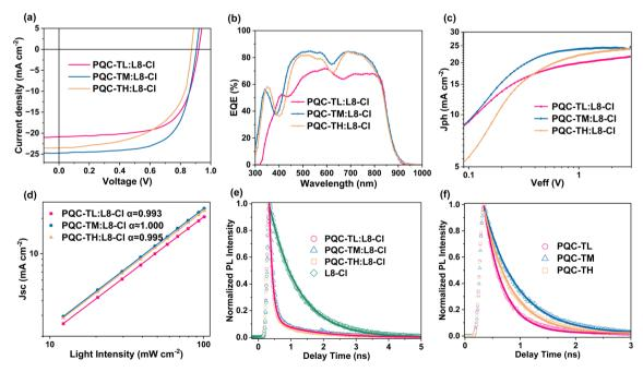
Fig. 2 (a) J-V characteristics, (b) EQE curves, (c)  $J_{ph}-V_{eff}$  curves, and (d) dependence of current density on light intensity of the OPVs based on PQC-TL:L8-Cl, PQC-TM:L8-Cl and PQC-TH:L8-Cl. (e) Time-resolved photoluminescence (TRPL) decay kinetics of PQC-TL:L8-Cl, PQC-TL:L TM:L8-CI, PQC-TH:L8-CI and L8-CI films excited at 550 nm. (f) TRPL decay kinetics of PQC-TL, PQC-TM, and PQC-TH neat films excited at 550 nm.
