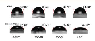
Fig. 4 Contact angle images of various films with water and diiodomethane droplets on top.
