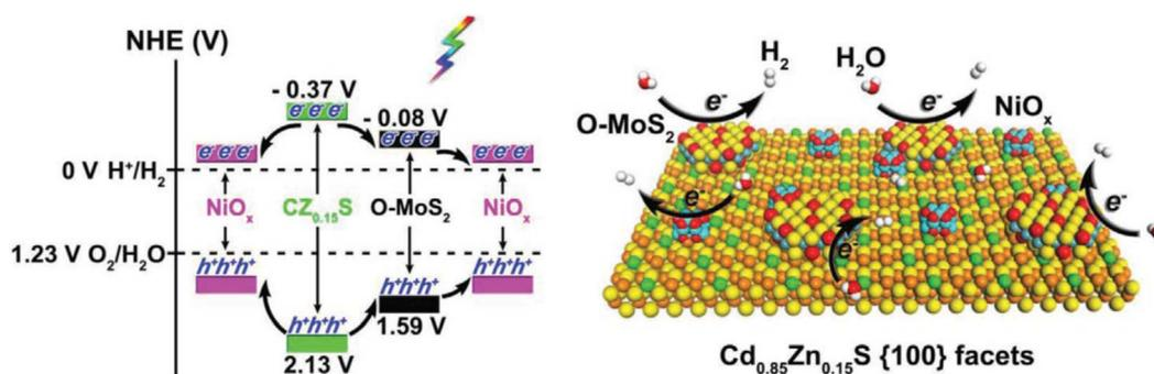
Fig. 10 Energy-band alignments of CZ<sub>0.15</sub>S, O-MoS<sub>2</sub>, and NiO<sub>x</sub> (left) and a schematic showing the photocatalytic hydrogen evolution over CZ<sub>0.15</sub>S@O-MoS<sub>2</sub>/NiO<sub>x</sub> (right image). Copyright 2019, Wiley-VCH.
