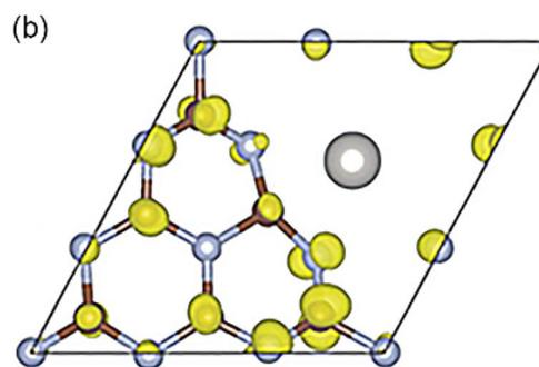
Fig. 2 (a) Energy-band alignment diagrams for g-C<sub>3</sub>N<sub>4</sub> and g-C<sub>3</sub>N<sub>4</sub>-Pt<sup>2+</sup>. (b) Photoexcited charge density transition from the Pt<sup>2+</sup>-induced hybrid highest occupied molecular orbital (HOMO) states to the lowest unoccupied molecular orbital (LUMO) of g-C<sub>3</sub>N<sub>4</sub>-Pt<sup>2+</sup>. Copyright 2016, Wiley-VCH.
