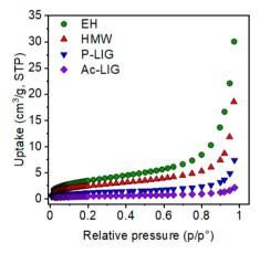
Fig. 2 Comparison between nitrogen adsorption isotherms collected at 77 K of HMW, EH, P\_LIG and Ac\_Lig.
