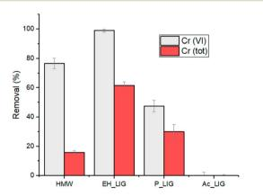
Fig. 8 Cr(tot) removal and Cr(vi) reduction by using different types of lignin at pH 2 (2 M HNO<sub>3</sub>). 1 g L<sup>-1</sup> of lignin; initial Cr(vi) concentration: 5  $mg L^{-1}$ ; contact time: 2 h.
