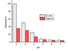
Fig. 3 Removal percentages of Cr(vi) and total chromium that remains in solution for experiments performed with an initial Cr(vi) concentration of 20 ppm; contact time: 24 hours; 1 g  $L^{-1}$  of HMW.
