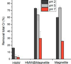
Fig. 10  $Cr(v_1)$  reduction (left) and total Cr removal (right) percentages for the experiments with HMW, magnetite and lignin@magnetite at three different pH values. pH controlled with 2 M HNO<sub>3</sub> or NaOH, 1 g L<sup>-1</sup> of lignin or lignin@magnetite and 0.43 g L<sup>-1</sup> of magnetite, an initial  $Cr(v_1)$  concentration of 5 mg L<sup>-1</sup>, and a contact time of 2 h.
