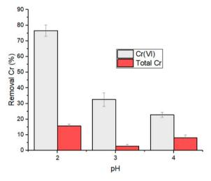
Fig. 4 Removal percentage of Cr(vi) and total chromium for experiments performed at 5 mg  $L^{-1}$  of initial  $Cr(v_1)$  concentration, 2 h contact time and 1 g  $L^{-1}$  of HMW.
