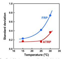
Fig. 8 The effect of the temperature on the standard deviation of  $\langle I \rangle_{\rm T}$  for the ATRP (red) and FRP (blue) gels. These gels were synthesized with a cross-linker content of 3 mol% at 25 °C.
