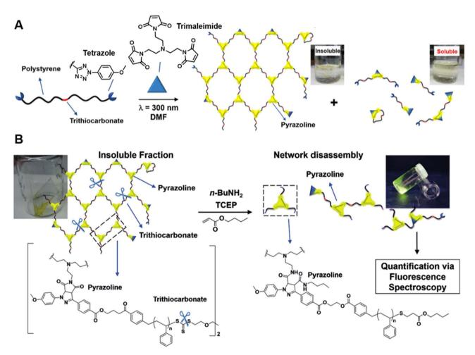
Fig. 7 (A) UV-induced NITEC crosslinking reaction between tetrazole chain-ends and trimaleimide cross-linkers, forming insoluble and soluble fractions. (B) Network disassembly *via* aminolysis. Determining the concentration of pyrazoline after aminolysis *via* fluorescence spectroscopy allows to quantify the number crosslinking points within the former network. Reproduced from ref. 191 with permission from Wiley, copyright 2018.
