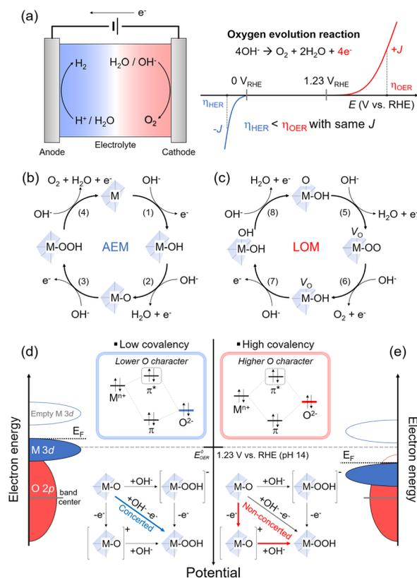
Fig. 2 Two principal OER processes. (a) Schematic illustration of the water splitting cell and  $I$ – $V$  curve for the HER and OER. Mechanism scheme of the 4-electron transferring oxygen evolution reaction by (b) the adsorbate evolution mechanism (AEM) and (c) lattice oxygen mediated (LOM) pathway. Schematic band diagram of (d) low covalent and (e) high covalent transition metal oxides. The concerted and non-concerted one-electron transfer processes are illustrated, respectively.
