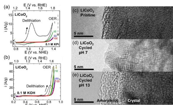
Fig. 4 Cyclic voltammogram (CV) of  $LiCoO_2$  (LCO) in (a) neutral and (b) alkaline electrolytes. (c–e) TEM image of LCO (c) pristine, (d) after cycling at pH 7, and (e) after cycling at pH 13. Adapted with permission from ref. 89. Copyright 2012 American Chemical Society.
