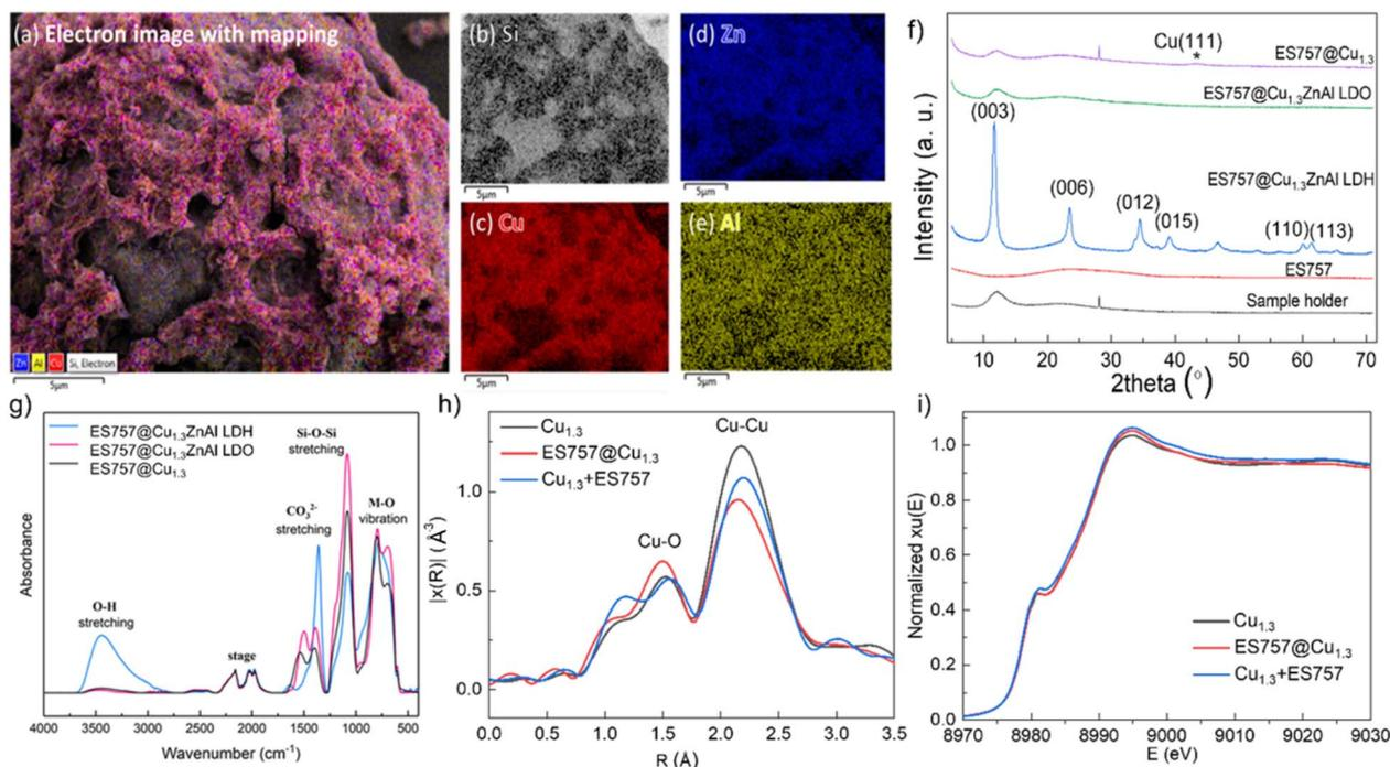
Fig. 2 Structural evolution during the preparation of ES757@Cu<sub>1.3</sub>. (a) Electron image with Zn, Al, Cu, Si element mapping; (b) Si; (c) Cu; (d) Zn; (e) Al of ES757@Cu<sub>1.3</sub>ZnAl LDH; (f) powder X-ray diffraction patterns; (g) FTIR spectra; (h) Fourier transformed magnitudes of the experimental Cu K-edge EXAFS spectra; (i) normalised Cu K-edge XANES spectra.
