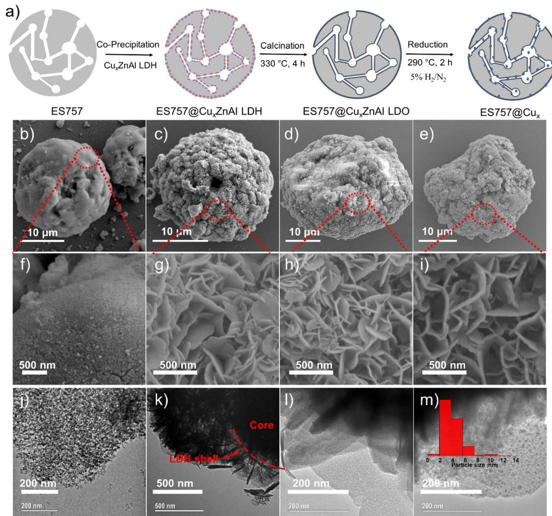
**Fig. 1** (a) Synthesis scheme of Cu nanoparticles from ES757@Cu<sub>x</sub>ZnAl LDH. SEM images of (b and f) ES757; (c and g) ES757@Cu<sub>1.3</sub>ZnAl LDH; (d and h) ES757@Cu<sub>1.3</sub>ZnAl LDO and (e and i) ES757@Cu<sub>1.3</sub>. TEM images of (j) ES757; (k) ES757@Cu<sub>1.3</sub>ZnAl LDH; (l) shell of ES757@Cu<sub>1.3</sub>ZnAl LDO; (m) shell of ES757@Cu<sub>1.3</sub>.
