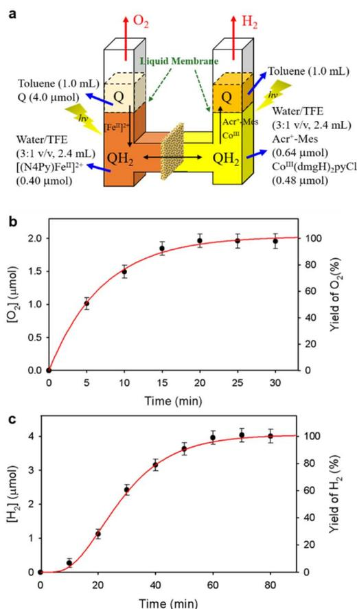
**Fig. 6** (a) A photocatalytic system used an H-type cell for the photocatalytic production of H<sub>2</sub> and O<sub>2</sub> from H<sub>2</sub>O. (b) Time profile of the production of O<sub>2</sub> in the photocatalytic H<sub>2</sub>O oxidation. (c) Time profile of the production of H<sub>2</sub> in the photocatalytic H<sub>2</sub>O reduction. Reprinted from ref. 90 with permission from American Chemical Society (Copyright 2022).
