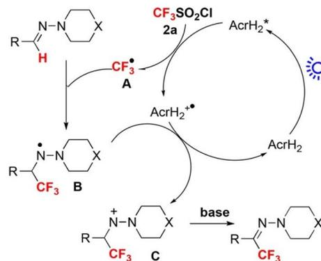
Scheme 1 Photocatalytic trifluoromethylation of hydrazones with an electrophilic  $\text{CF}_3$ -transfer reagent ( $\text{CF}_3\text{SO}_2\text{Cl}$ ) by  $\text{AcrH}_2$  photoredox catalysis. Reprinted from ref. 29 with permission from John Wiley and Sons (Copyright 2017).
