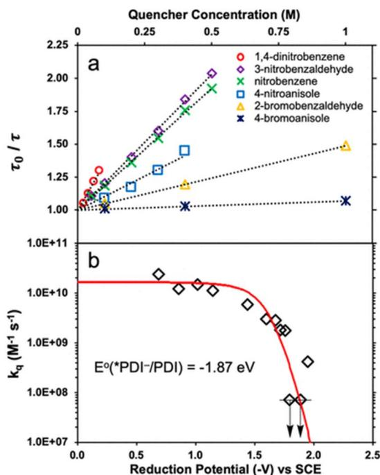
**Fig. 1** (a) Stern-Volmer plots for lifetime quenching of \*PDI<sup>•-</sup> versus concentrations of electron acceptors. (b) Dependence of logarithm of  $k_q$  of electron transfer from \*PDI<sup>•-</sup> to electron acceptors on the 1 e<sup>-</sup> reduction potentials ( $E_{\text{red}}$  vs. SCE) of electron acceptors. Red line represents the fit calculated using the Rehm-Weller equation. Reprinted from ref. 39 with permission from American Chemical Society (Copyright 2020).
