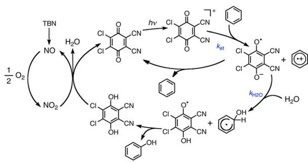
Scheme 7 A mechanism for photohydroxylation of benzene by dioxygen with DDQ used as a photoredox catalyst in the presence of TBN and  $\text{H}_2\text{O}$  in MeCN under photoirradiation. Reprinted from ref. 44 with permission from American Chemical Society (Copyright 2013).
