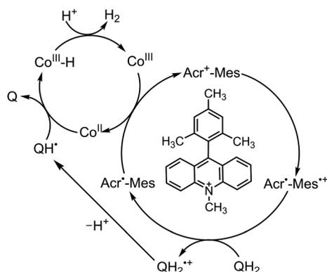
**Scheme 14** Proposed PS-I model mechanism of photocatalytic H<sub>2</sub> evolution from hydroquinone (QH<sub>2</sub>) derivatives with Acr<sup>+</sup>-Mes and Co<sup>III</sup> complex. Reprinted from ref. 87 with permission from American Chemical Society (Copyright 2020).
