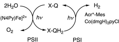
**Scheme 15** A scheme for the photocatalytic production of H<sub>2</sub> and O<sub>2</sub> from H<sub>2</sub>O by the combination of the molecular models of PS-I and PS-II with use of X-Q/X-QH<sub>2</sub> as plastoquinone/plastoquinol analogue in photosynthesis. Reprinted from ref. 90 with permission from American Chemical Society (Copyright 2022).
