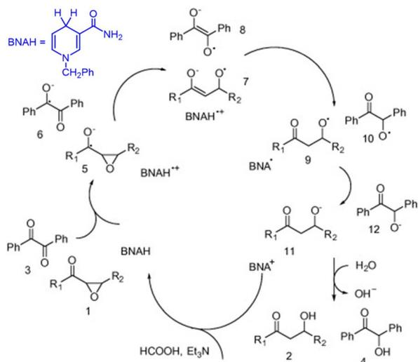
**Scheme 3** Photocatalytic hydrogenation of  $\alpha,\beta$ -epoxy ketones to  $\beta$ -hydroxy ketones with  $\text{HCO}_2\text{H}$  and  $\text{Et}_3\text{N}$  by BNAH photoredox catalysis. Reproduced from ref. 33 with permission from American Chemical Society (Copyright 2006).
