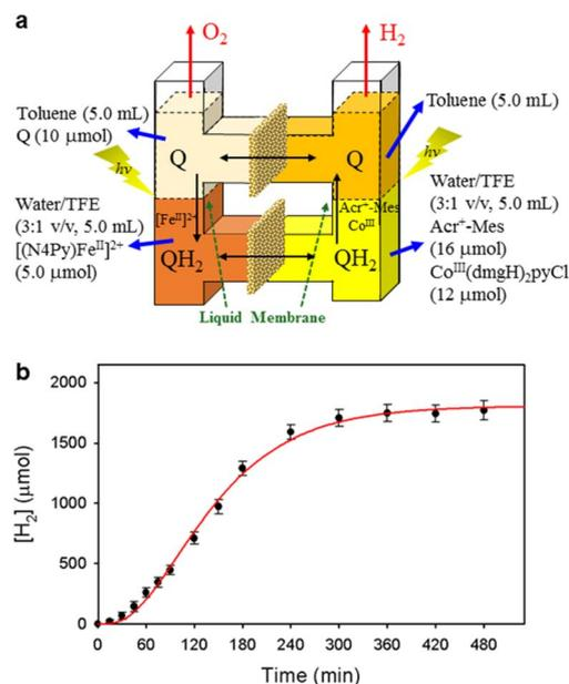
**Fig. 7** (a) A photochemical cell used for photocatalytic production of H<sub>2</sub> and O<sub>2</sub> from H<sub>2</sub>O. (b) Time profile of the production of H<sub>2</sub> in the photocatalytic H<sub>2</sub>O splitting under photoirradiation. Reprinted from ref. 90 with permission from American Chemical Society (Copyright 2022).
