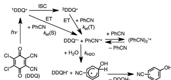
Scheme 8 Proposed mechanism for photohydroxylation of benzonitrile with DDQ and  $\text{H}_2\text{O}$  in MeCN via  $^1\text{DDQ}^*$ . Reprinted from ref. 47 with permission from John Wiley and Sons (Copyright 2015).
