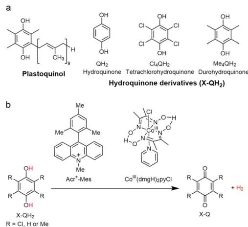
**Scheme 13** (a) Plastoquinol and its analogs.<sup>84</sup> (b) Photocatalytic hydrogen evolution using the PS-I model system consisting of hydroquinone derivatives, 9-mesityl-10-methylacridinium ion as a PRC model and  $Co^{III}(dmgH)_2pyCl$ . Reprinted from ref. 87 with permission from American Chemical Society (Copyright 2020).
