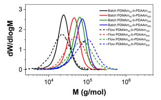
Fig. 7 Molecular weight distributions of PDMAm<sub>40</sub>-b-PDAAm<sub>m</sub> copolymers prepared simultaneously in batch and a miniature CSTR cascade for a reaction time of 50 minutes at 70 °C. The same batch synthesised PDMAm<sub>40</sub> macro-CTA was used in each case. [CTA]: [initiator] = 10:1.
