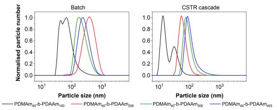
Fig. 8 Particle size distributions of PDMAm<sub>40</sub>-b-PDAAm<sub>m</sub> copolymers prepared simultaneously in batch (left) and a miniature CSTR cascade (right) for a reaction time of 50 minutes at 70 °C. The same batch synthesised PDMAm<sub>40</sub> macro-CTA was used in each case. [CTA]: [initiator] = 10:1.
