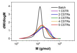
Fig. 5 MWDs for different CSTR cascade configurations versus the batch MWD for the aqueous solution RAFT polymerisation of 30% w/w PDMAm $_{100}$  at 80 °C. Average reaction/residence time = 25 minutes. [CTA]:[initiator] = 10:1.
