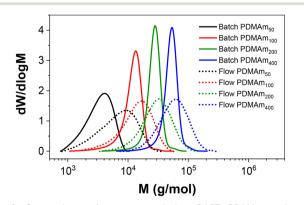
Fig. 4 Comparison of aqueous solution RAFT PDMAm polymers prepared in batch versus continuous-flow in a miniature CSTR cascade. All polymers were prepared at 30% w/w, 80 °C, 25 minutes.
