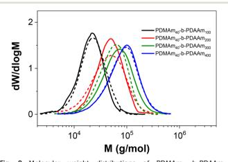
Fig. 9 Molecular weight distributions of PDMAm<sub>40</sub>-b-PDAAm<sub>m</sub> copolymers prepared in a miniature CSTR cascade using a batch macro-CTA (solid lines) versus a telescoped configuration with macro-CTA prepared inline using a tubular reactor (dashed lines). PDMAm<sub>40</sub> macro-CTA was prepared at 80 °C for 40 minutes, copolymerisation at 70 °C for 50 minutes. [CTA]: [initiator] = 10:1.
