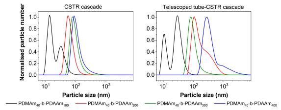
Fig. 10 Particle size distributions of PDMAm<sub>40</sub>-b-PDAAm<sub>m</sub> copolymers prepared via RAFT dispersion polymerisation in a miniature CSTR cascade using a batch macro-CTA (left) versus in a miniature CSTR cascade with a macro-CTA prepared upstream in a telescoped tubular reactor (right). PDMAm<sub>40</sub> macro-CTA was prepared at 80 °C for 40 minutes, with copolymerisation at 70 °C for 50 minutes. [CTA]: [initiator] = 10:1.
