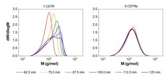
Fig. 6 MWDs obtained at different time points for the aqueous solution RAFT polymerisation of DMAm at 80 °C in either one (left) or five (right) CSTRs. Average residence time of 25 minutes, [CTA]: [initiator] = 10:1.
