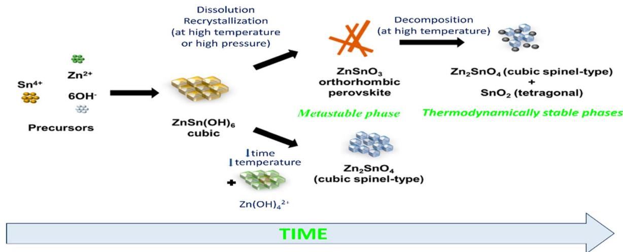
Fig. 1 Schematic illustration of phase rearrangements during the hydrothermal process of zinc stannate nanostructures as a function of reaction energy and synthesis time.<sup>34</sup>
