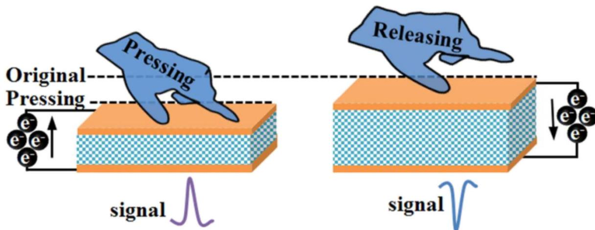
Fig. 23 Working mechanism of generating power from a piezoelectric nanogenerator.<sup>215</sup>
