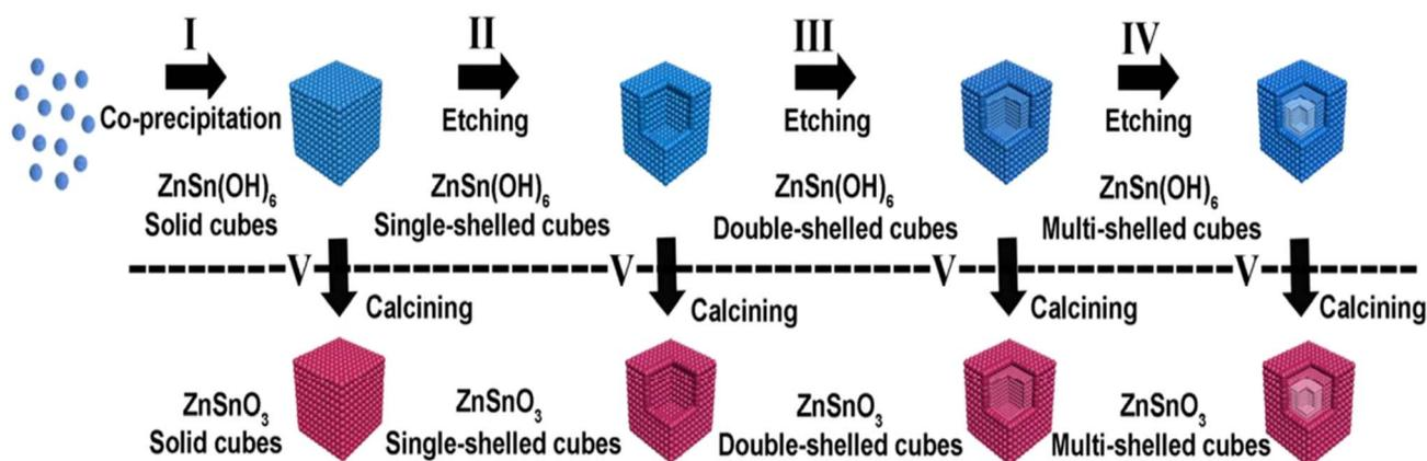
Fig. 15 Schematic illustration of the fabrication of ZnSnO<sub>3</sub> hollow-boxes under basic-etching and calcination.<sup>129</sup>
