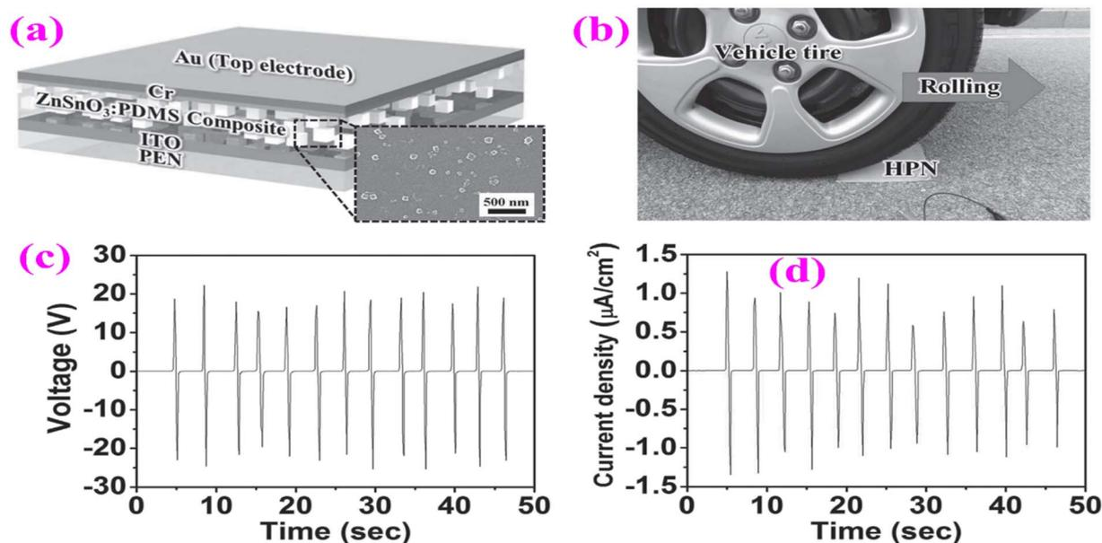
Fig. 22 Structure and power generation by HP-NG when a tire is rolled. (a) Illustration of the structure of the ZnSnO<sub>3</sub>:PDMS nanocomposite-based flexible HP-NG as seen by the cross-sectional FESEM image. (b) Experimental setup for power production under the rolling of a vehicle tire, in which ZnSnO<sub>3</sub>:PDMS HP-NG was attached to the road. (c) Output voltage and (d) current density from HP-NG induced by the loading and unloading of a vehicle tire.<sup>214</sup>
