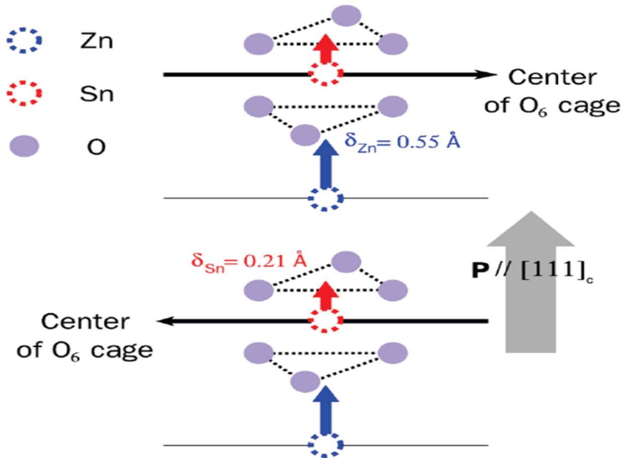
Fig. 4 Ionic rearrangements of Zn and Sn in the  $R3c$  phase of  $ZnSnO_3$ .<sup>49</sup>
