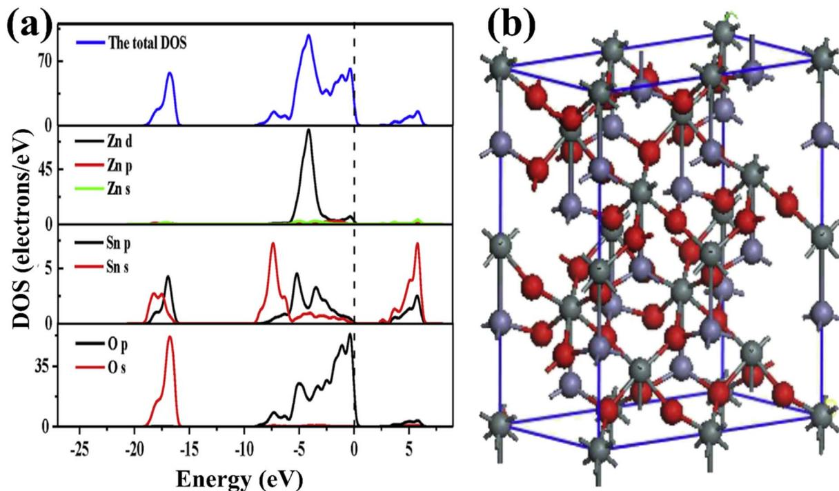
Fig. 6 (a) DOS and PDOS for ZnSnO<sub>3</sub>. (b) Supercells of Zn<sub>12</sub>Sn<sub>12</sub>O<sub>36</sub>.<sup>69</sup>
