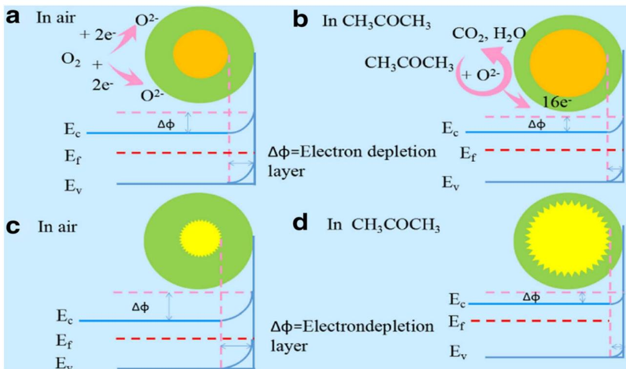
Fig. 18 Schematic band diagrams of ZnSnO<sub>3</sub> hollow microspheres exposed to (a) air and (b) CH<sub>3</sub>COCH<sub>3</sub>, and ZnSnO<sub>3</sub>/SnO<sub>2</sub> hollow urchin gas sensors exposed to (c) air and (d) CH<sub>3</sub>COCH<sub>3</sub>.<sup>218</sup>
