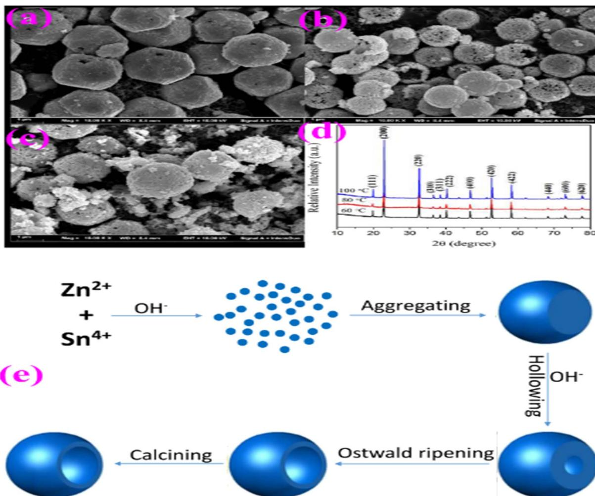
Fig. 14 SEM images of  $\text{ZnSnO}_3$  obtained at different reaction temperatures: (a) 60 °C, (b) 80 °C, and (c) 100 °C. (d) XRD patterns of  $\text{ZnSn(OH)}_6$  precursor. (e) Schematic illustration of the possible formation mechanism of  $\text{ZnSnO}_3$  hollow spheres.<sup>70</sup>
