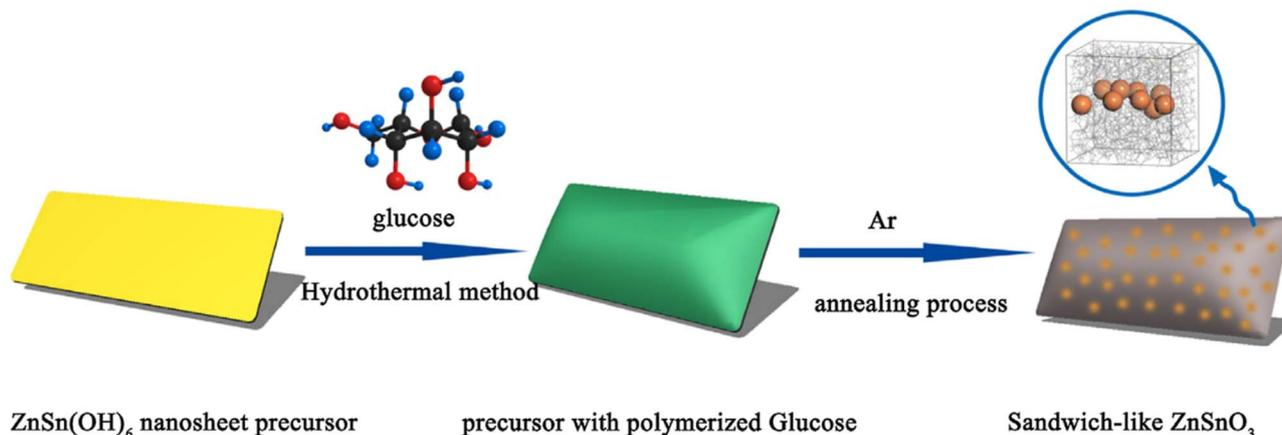
Fig. 19 Schematic illustration depicting the synthesis of sandwich-like ZnSnO<sub>3</sub>@C.<sup>194</sup>
