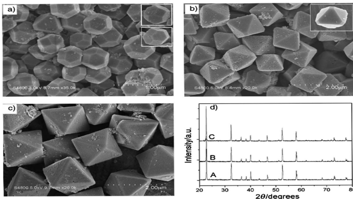
Fig. 11 SEM micrograph of  $\text{ZnSnO}_3$  obtained using: (a) SDBS 0.15 M, (b) SDBS 0.4 M, and (c) SDBS 0.75 M. (d) XRD pattern of (A) 14-faceted polyhedra, (B) truncated octahedra and (C) octahedra.<sup>102</sup>
