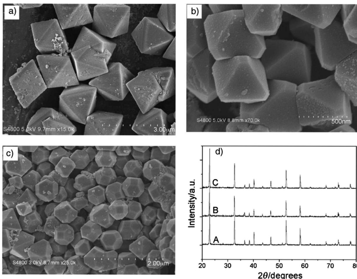
Fig. 12 Typical SEM images of the as-prepared  $\text{ZnSnO}_3$  products: (a) CTAB 0.15 M, (b) CTAB 0.4 M, and (c) CTAB 0.75 M. (d) Corresponding XRD patterns of the as-prepared  $\text{ZnSnO}_3$  polyhedra, (A) octahedra, (B) truncated octahedra and (C) 14-faceted polyhedra.<sup>102</sup>
