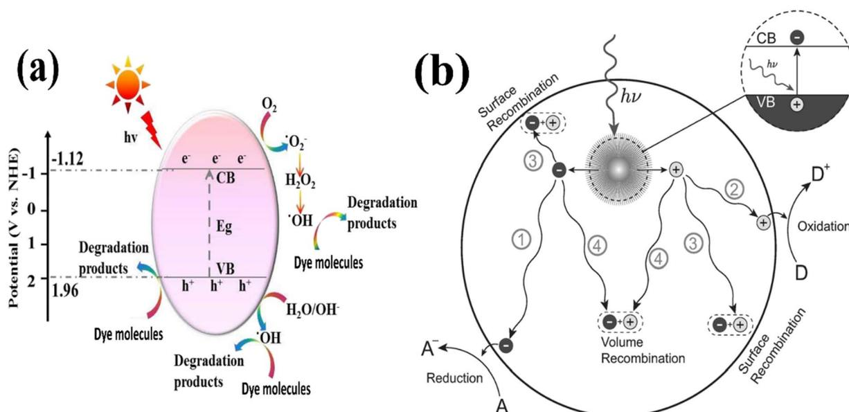
Fig. 17 Illustration of (a) photocatalytic mechanism. (b) Photoinduced formation of an electron hole pair in a semiconductor.<sup>148,217</sup>
