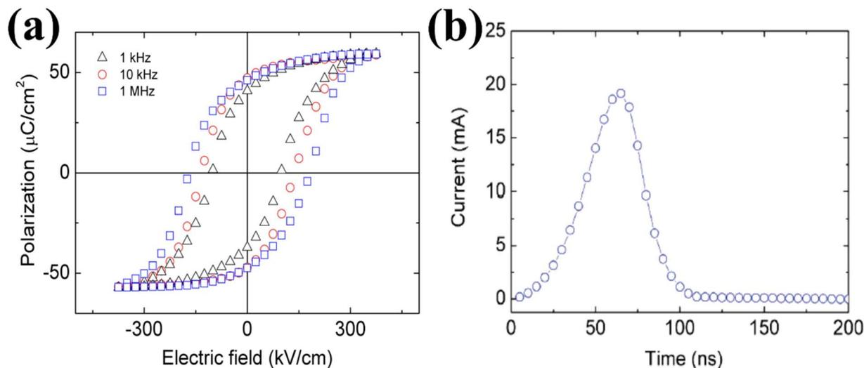
Fig. 3 (a) Hysteresis loops of the Pt/ZnSnO<sub>3</sub>/SrRuO<sub>3</sub> capacitor observed at different measurement frequencies. (b) Switching-current as a bias of 5 V. The fast-switching behaviour is within 100 ns.<sup>49</sup>
