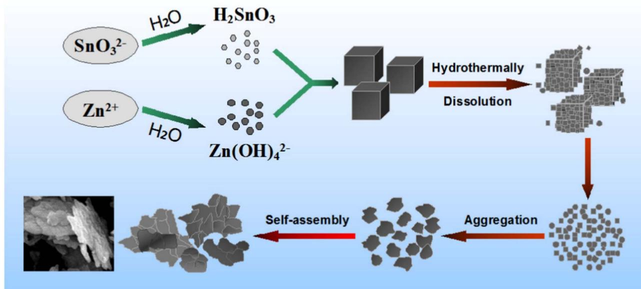
Fig. 10 Diagram depicting the probable process for the formation of the precursor  $\text{ZnSn(OH)}_6$ .<sup>95</sup>
