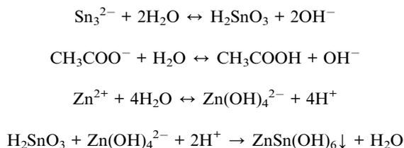
Under hydrothermal conditions, the metastable  $\text{ZnSn}(\text{OH})_6$  nanocubes will undergo decomposition and subsequent recrystallization as the temperature and pressure increases. This process follows the breaking-recrystallization pathway, resulting in the formation of a stable nanostructure. Fig. 10 depicts the hypothetical growth process graphically.
