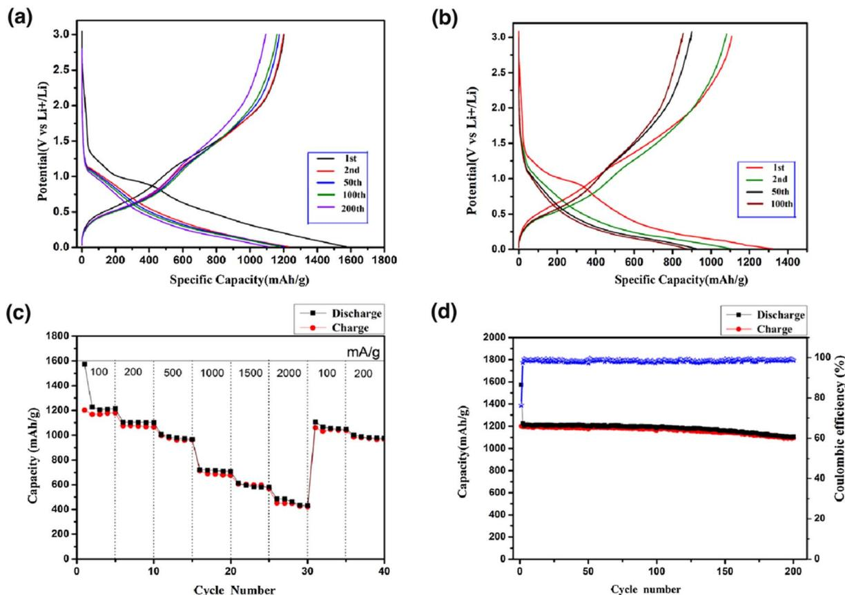
Fig. 20 Charge–discharge profiles of (a) sandwich-like  $\text{ZnSnO}_3\text{@C}$  and (b) sheet-like  $\text{ZnSnO}_3$  at  $100 \text{ mA g}^{-1}$ . (c) Cycling activity at various current densities. (d) Cycling activity at  $100 \text{ mA g}^{-1}$  of the sandwich-like  $\text{ZnSnO}_3\text{@C}$ .<sup>194</sup>
