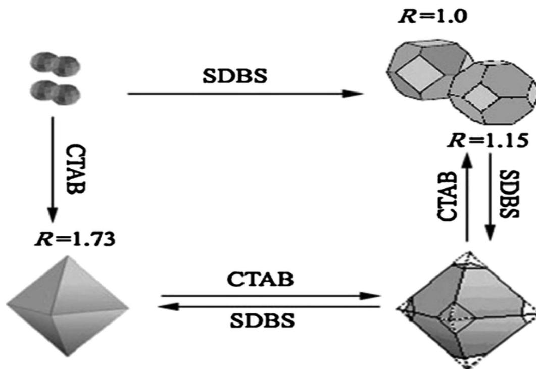
Fig. 13 Schematic diagram depicting the relationship between the ratio  $R$  and the transformation of the crystal shape.<sup>102</sup>
