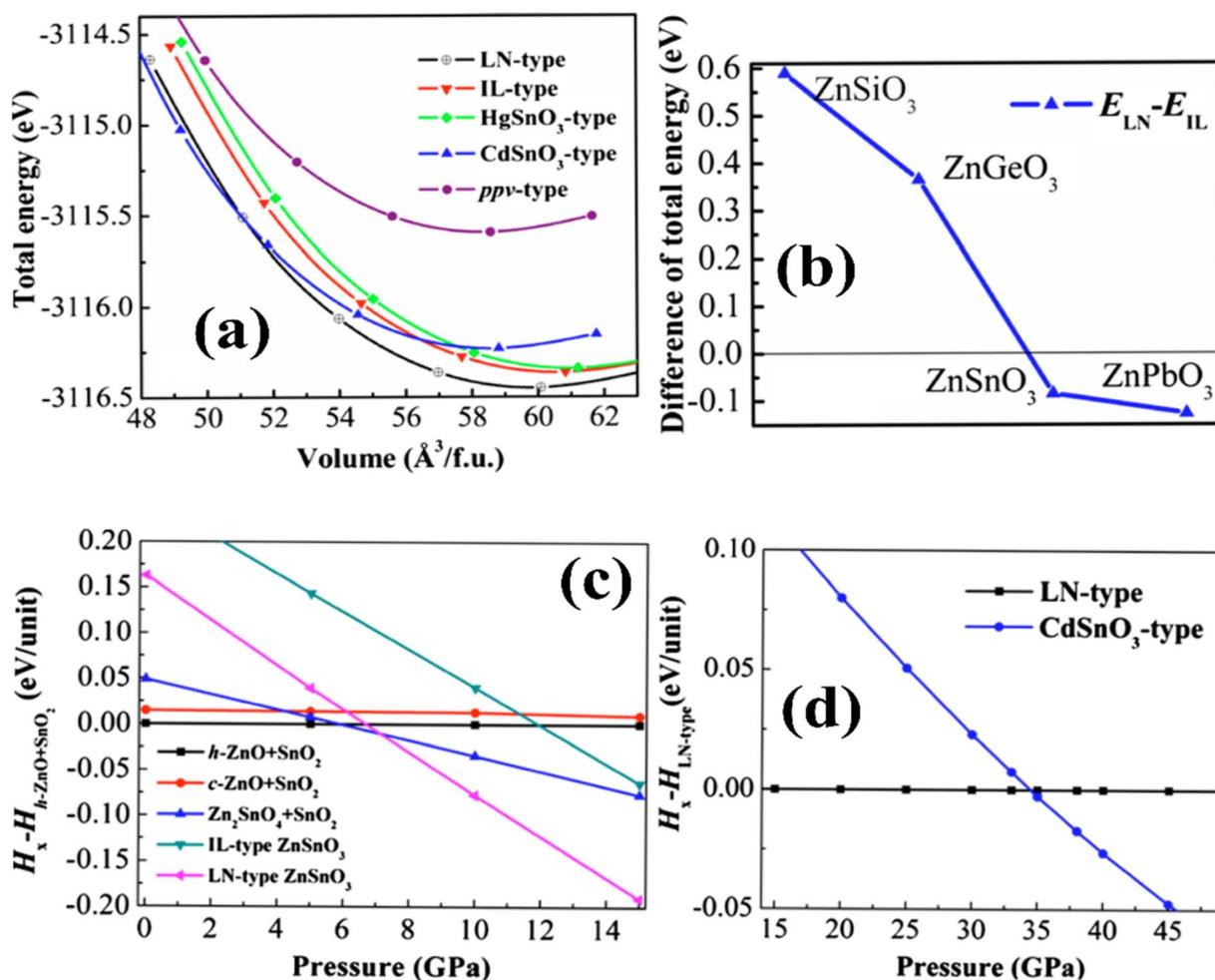
Fig. 5 (a)  $E$ - $V$  curve for six feasible phases. (b) Energy variation in  $ZnXO_3$ . (c) Enthalpy variation among heterogenous component oxides. (d) Enthalpy variation in LN-type and  $CdSnO_3$ -type phases.<sup>65</sup>
