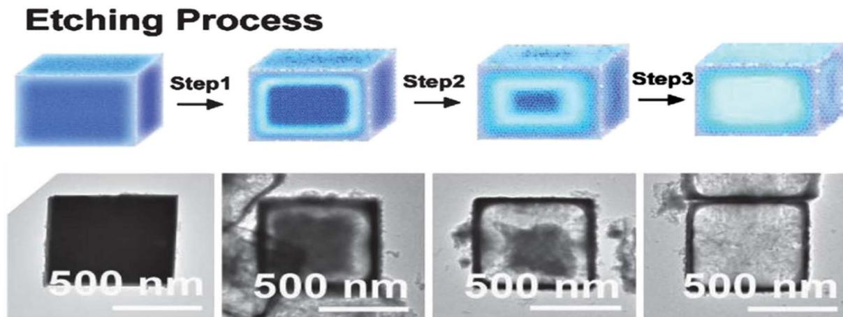
Fig. 16 Potential mechanism illustrating the acid etching process and the resulting synthesized products when employing cubic  $\text{ZnSnO}_3$  templates.<sup>92</sup>
