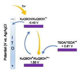
Fig. 8 Proposed mechanism for anodic photocurrent generation of KuQ9OH|ITO/H<sub>2</sub>O/Na<sub>2</sub>SO<sub>4</sub> 0.1 M/TEOA 50 mM.
