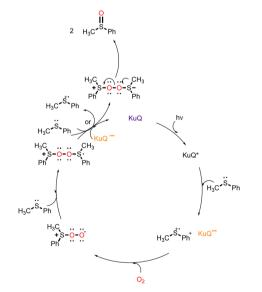
$\begin{array}{lll} \textbf{Scheme 5} & \textbf{Proposed} & \textbf{mechanism} & \textbf{for thioether photooxidation} \\ \textbf{promoted by KuQ}. \end{array}$
