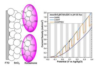
Fig. 14 LSV of KuQ3CO<sub>2</sub>H|meso-SnO<sub>2</sub> in aqueous ascorbate buffer pH 5.8, 20 mV s $^{-1}$ , light: AM 1.5G + 400 nm cut-off filter. Reproduced from ref 87
