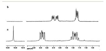
Fig. 4 Comparison between H-NMR spectra of KuQTEGMe in (a) CDCl<sub>3</sub>, (b) DMSO-d<sub>6</sub>. Reprinted with permission from ref. 27. Copyright 2017 American Chemical Society.
