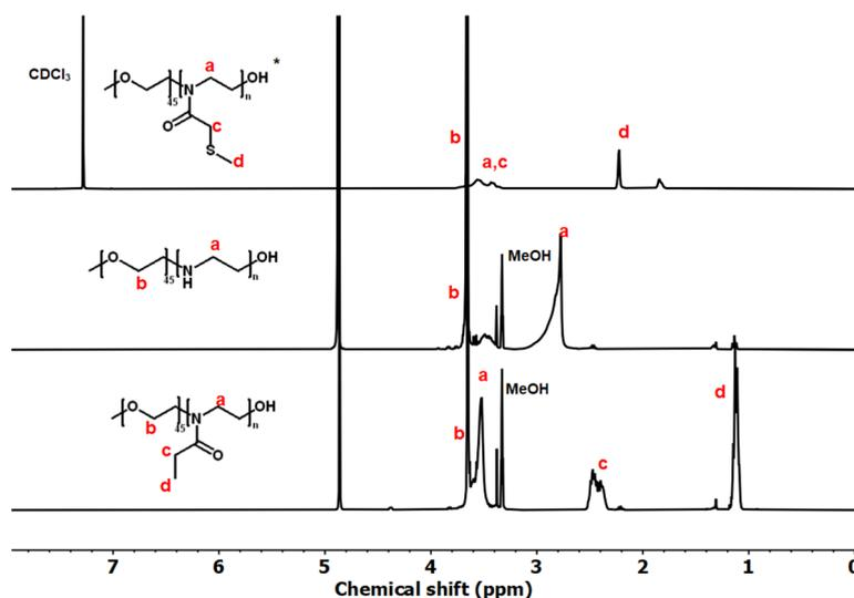
**Fig. 4** <sup>1</sup>H NMR spectra of PEG-*b*-PMTMeOx in CDCl<sub>3</sub>; and PEG-*b*-PEI and PEG-*b*-PEtOx, in CD<sub>3</sub>OD (\*some -OH groups were transformed into their respective esters).
