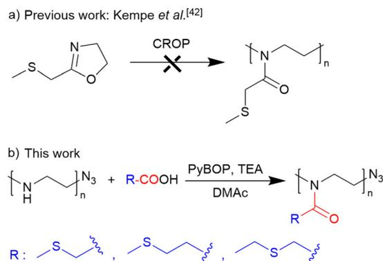
**Scheme 1** (a) Schematic representation of the unsuccessful CROP of 2-methylthiomethyl-2-oxazoline<sup>42</sup> and (b) synthesis of thioether-containing homopolymers *via* acylation of well-defined PEI.
