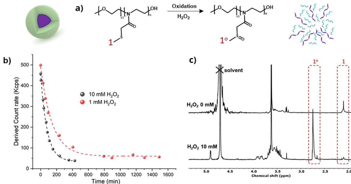
**Fig. 7** (a) Schematic illustration of the oxidative reaction of PEG-*b*-PMTMeOx (DP = 30) block copolymer NPs with H<sub>2</sub>O<sub>2</sub>, (b) decrease of DLS scattering light intensity of the nanoparticle solution at 1 mg mL<sup>-1</sup> when adding 1 and 10 mM H<sub>2</sub>O<sub>2</sub> and (c) <sup>1</sup>H NMR spectra of PEG-*b*-PMTMeOx before and 24 hours after oxidation with 10 mM H<sub>2</sub>O<sub>2</sub> in D<sub>2</sub>O.
