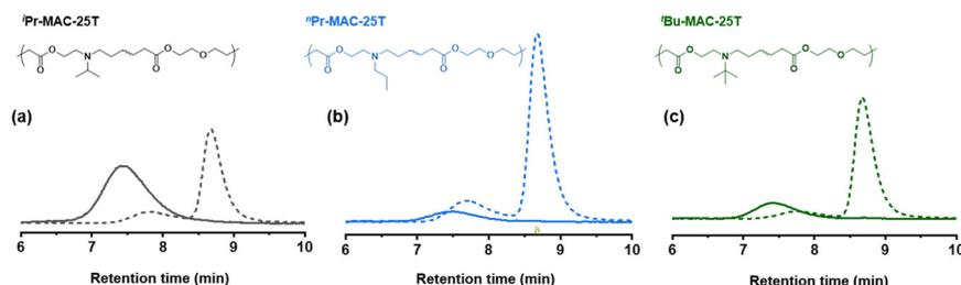
**Fig. 4** SEC analysis of copolymers before (solid lines) and after hydrolytic degradation (dashed lines) under accelerated conditions. Light scattering signals of (a) <sup>i</sup>Pr-MAC-25T, (b) <sup>n</sup>Pr-MAC-25T and (c) <sup>t</sup>Bu-MAC-25T are depicted.
