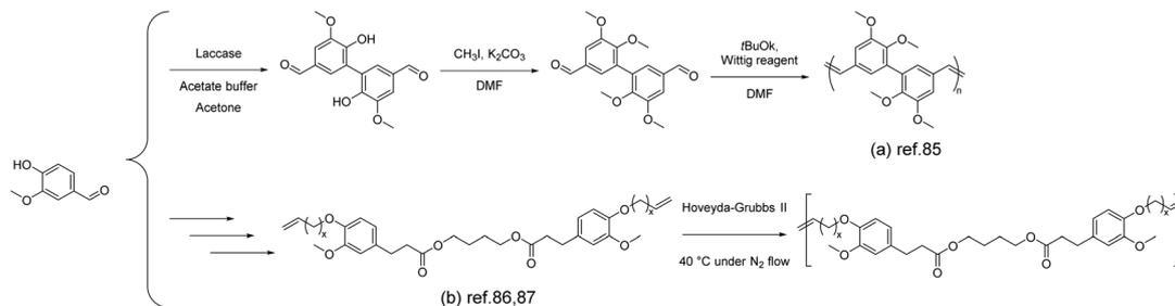
**Scheme 9** The synthesis of vanillin-derived unsaturated polyolefins by ADMET polymerization: (a) Reproduced from ref. 85 with permission from the Royal Society of Chemistry, copyright 2015. (b) Reproduced from ref. 86 with permission from Elsevier, copyright 2015 and reproduced from ref. 87 with permission from the Royal Society of Chemistry, copyright 2013.
