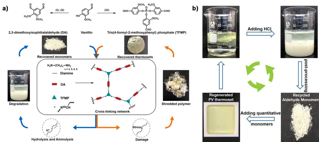
**Fig. 3** (a) Synthetic route and reprocessing of the fully bio-based vitrimers. (b) Digital photographs of the chemical recycling process of PV-NDA-25 through the recovered monomer. Reproduced from ref. 114 with permission from the American Chemical Society, copyright 2022.
