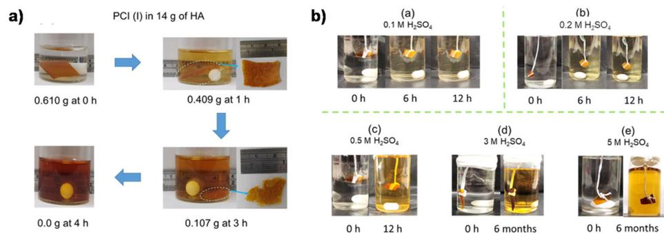
**Fig. 5** (a) Digital photographs of degradation of PCI (I) by HA. (b) Digital photographs of acid hydrolysis experiments of PCI (I) at different concentrations: (a) 0.1 M, (b) 0.2 M, (c) 0.5 M, (d) 3 M, and (e) 5 M H<sub>2</sub>SO<sub>4</sub> in 30 mL of THF/H<sub>2</sub>O (v/v, 8/2) at 50 °C. Reproduced from ref. 116 with permission from the American Chemical Society, copyright 2023.
