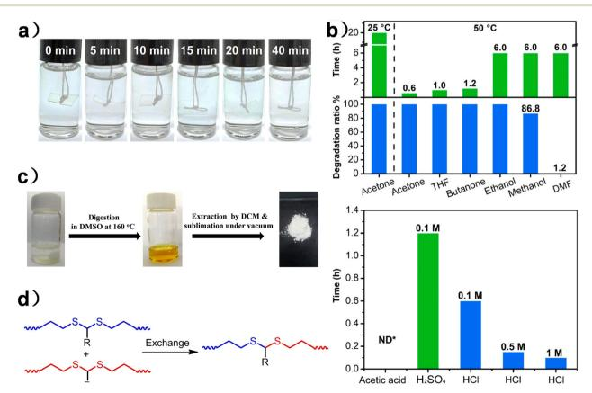
Fig. 8 (a) Degradation process of PU-HMDO at different times in a 0.1 M HCl  $H_2$ O/acetone (1/9, v/v) solution. (b) Degradation of PU-HMDO under different conditions. Reproduced from ref. 125 with permission from the American Chemical Society, copyright 2020. (c) Polythioacetals in DMSO before and after thermal treatment at 160 °C for 12 hours. (d) Schematic illustration of dynamic exchanges between dithioacetals. Reproduced from ref. 126 with permission from John Wiley & Sons, copyright 2023.
