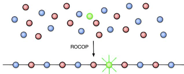
**Fig. 1** Chromophore-doped polymers *via* ring-opening copolymerization (ROCOP).
