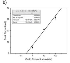
Fig. 6 (a) DPV response curves for polydopamine entrapped F8 sensor in increasing concentrations of copper from 0 to 100  $\mu M$ . All measurements were taken in PBS after 15 min with stirring (100 rpm). (b) Peak current measured in sensing range of -0.4 V to 0.1 V for different copper concentrations with a linear fit after subtracting a baseline taken in PBS only.
