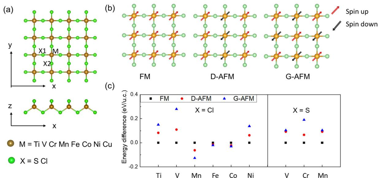
**Fig. 1** Structure and magnetic states of monolayer MX. (a) Overview and sideview of monolayer MX, where the dark yellow and the green balls indicate the transition metal atoms and sulfur or chlorine, respectively. (b) Schematic top view of three possible magnetic orders of MX: FM order, checkerboard AFM order and collinear AFM order. The red and black arrows represent the up and down spins of transition metal atoms, respectively. (c) The magnetic order in the ground state of MX.
