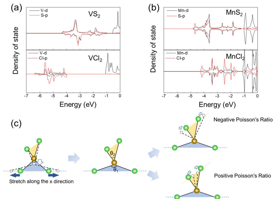
**Fig. 3** Deformation mechanism. (a) DOS of VS<sub>2</sub> (upper panel) and VCl<sub>2</sub> (lower panel), (b) DOS of MnS<sub>2</sub> (upper panel) and MnCl<sub>2</sub> (lower panel), where the blue, black and red lines indicate the s and d orbitals of V/Mn atoms, and p orbital of S/Cl atoms, respectively. (c) Deformation mechanism of MX, where the grey and cyan arrows indicate the movement of X atom and M atom, respectively.
