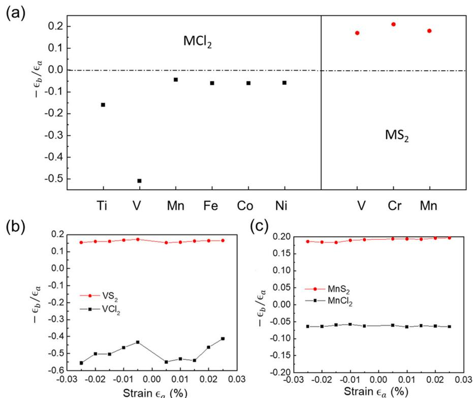
**Fig. 2** Auxetic effect. (a)  $-\epsilon_b/\epsilon_a$  of  $\text{MX}_2$ , where the black and red dots indicate  $\text{MCl}_2$  and  $\text{MS}_2$ , respectively. (b)  $-\epsilon_b/\epsilon_a$  of  $\text{VCl}_2$  and  $\text{VS}_2$  with the strain range from  $-2.5\%$  to  $2.5\%$ . (c)  $-\epsilon_b/\epsilon_a$  of  $\text{MnCl}_2$  and  $\text{MnS}_2$  with the strain range from  $-2.5\%$  to  $2.5\%$ .
