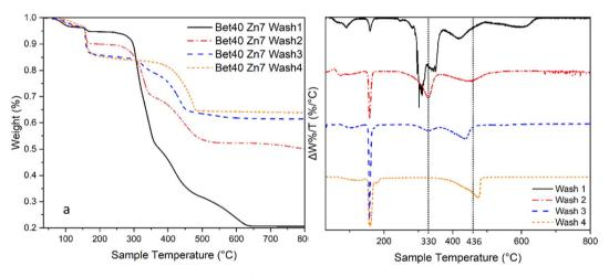
Fig. 16 In this two part figure, illustrating the same data the TGA curve is shown on the left and the first derivative of mass loss plot with different washing times is shown on the right.
