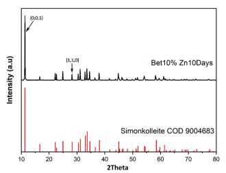
Fig. 4 The XRD patterns of the JCPDS standard peak of simonkolleite (COD 9004683) (bottom diffraction pattern shown in red) and the synthesised product recovered from 10% of betaine · HCl after a 10 day reaction period (top diffraction pattern shown in black).
