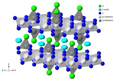
Fig. 1 The layered double hydroxide crystal structure of simonkolleite. 15,60 Zinc containing octahedron and tetrahedrons are shown (light and dark grey, respectively) with the interlayer spacing containing water. N. b. H atoms are not shown.
