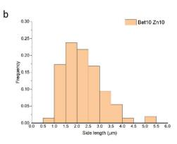
Fig. 5 (a) SEM images of product simonkolleite; (b) particles size distribution for the case of 10% of betaine HCl with a 10 day reaction. (b) The sample presented is for n=200, where hexagonal crystals showed regularity (i.e. regular hexagons). The distribution step-size selected is  $0.5 \, \mu m$ , based on measurement confidence.
