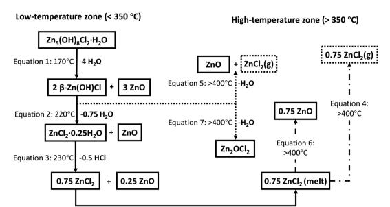
Fig. 15 Schematic of a series of reaction equations for the decomposition process of simonkolleite; the residual substances are represented in the solid box, and volatile substances are represented by the dashed box. The arrows represent the reaction direction of the thermal decomposition process, and the solid arrows represent the most likely reactions.<sup>45,62,63</sup>
