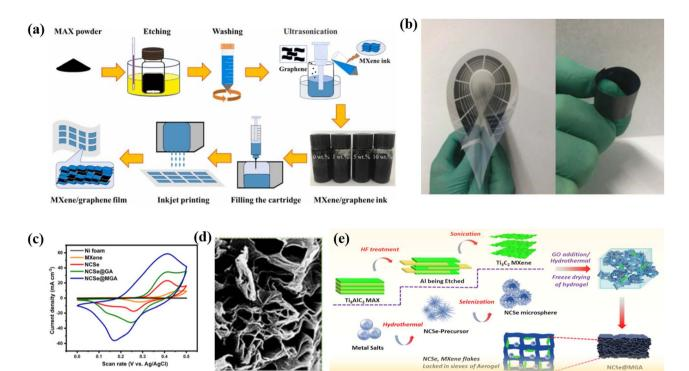
Fig. 5 (a) A diagram showing the process of inkjet printing of MXene/graphene films, (b) the images of a flexible MXene/graphene composite electrode fabricated by inkjet printing process, (c) comparison of CV curves, (d) the interlinked network of NCSe@GA, and (e) a schematic representation of the production of Ti<sub>3</sub>C<sub>2</sub> MXene, NCSe microspheres, and the creation of NCSe@MG.
