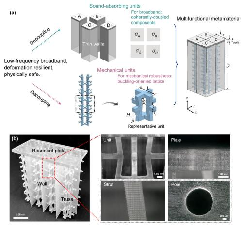
Fig. 2 Specific decoupled design procedures for our DPMM and the 3D-printed specimen. (a) Demonstration of the decoupled design for an engineered multifunctional metamaterial. Based on the desired properties, the acoustic and mechanical units are designed independently. (b) One representative DPMM specimen with microstructural characteristics: the re-entrant unit, resonant plate, strut, and micro-perforation.
