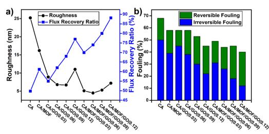
Fig. 7 (a) Influence of MOF and GO dosing on cellulose acetate membrane on surface roughness and flux recovery ratio; (b) effect of MOF and GO dosing on cellulose acetate membrane on the antifouling performance (reversible and irreversible fouling).<sup>144</sup>
