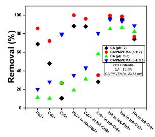
Fig. 10 Influence of pH, polymer composition, and addition of negatively-charged organic compound on removal rate of three heavy metals (Pb<sup>2+</sup>, Cd<sup>2+</sup>, and Cr<sup>6+</sup>).<sup>251</sup> (Metal ion concentration = 10 ppm, Humic acid = 20 ppm, pressure = 4 bar, contact time = 2 h, rotation speed = 300 rpm, and Temperature = 25 °C).
