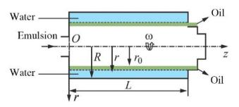
Fig. 14 Schematic for calculating the oil-in-water emulsion separation process in the bowl of a continuous centrifuge. This figure is adopted from ref. 145 with permission
