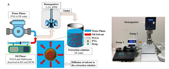
Fig. 6 Utilizing in-line homogenization in the emulsion solvent extraction/evaporation process for producing drug-loaded PLGA particles. (a) Schematic of naltrexone-loaded PLGA generation using an in-line emulsification-extraction process. (b) Experimental set-up used to generate particles by pumping both oil- and aqueous-phases into the homogenizer and transferring the emulsion to the extraction solution. The figure is adopted from ref. 54 with permission
