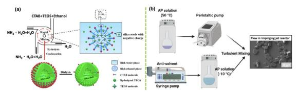
Fig. 8 (a) Production of MSNs by flash technology (adopted from ref. 94 with permission). (b) Flash technology system for the fabrication of ammonium perchlorate particles (adopted from ref. 86 with permission)
