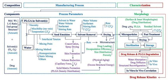
Fig. 5 A flow chart of manufacturing PLGA microparticles by emulsion methods and the parameters affecting the properties of the formulation. Each color represents specific parameters or processes: Dark blue for components, dark blue in a box for main processes, blue for process parameters, purple for physicochemical processes, green for microparticle properties for characterization, and red for drug release characterization. The figure is adopted from ref. 45 with permission.
