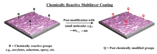
Fig. 4 Schematic representation of chemical modification of the 'reactive' covalently crosslinked multilayer coating
