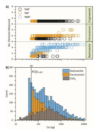
Fig. 3 Comparison of particle classification from the first SSML model to the mass distribution of Ce. (A) Individual particle events are plotted by the number of elements detected and grouped vertically by the true particle class as a function of Ce mass (ag). Bubbles are colored by the predicted classification. (B) The mass distribution of each of the three pristine samples; the vertical line indicates  $X_{C,sp,Ce,INP}^{mass}$
