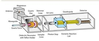
Fig. 1 Schematic depiction of the MICAP-MS.
