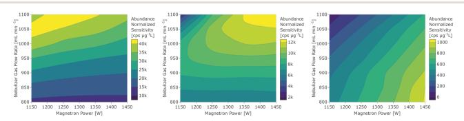
Fig. 2 The abundance normalized sensitivity of an analyte is shown in dependence of the operating power and the nebulizer gas flow rate as contour plots. Three different behaviours exist and are represented with <sup>133</sup>Cs (left), <sup>59</sup>Co (middle) and <sup>75</sup>As (right), measured in the standard interface & additional pump configuration.
