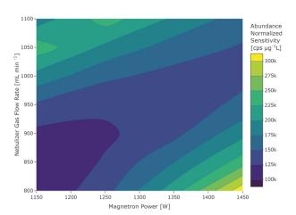
Fig. 3 The operating power vs. gas flow rate contour plot shows two maxima for the sensitivity of <sup>40</sup>Ca in the standard interface θ pump configuration, which can be accounted to an argon interference at high operating powers and low gas flow rates and the actual calcium at low operating powers and high gas flow rates.
