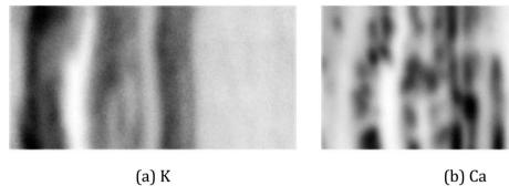
Fig. 7 Shift corrected means of  $\mu$ -XRF scans (with n=48 scans) of the element potassium (a) and calcium (b); calculated by graph registration, with d=20.
