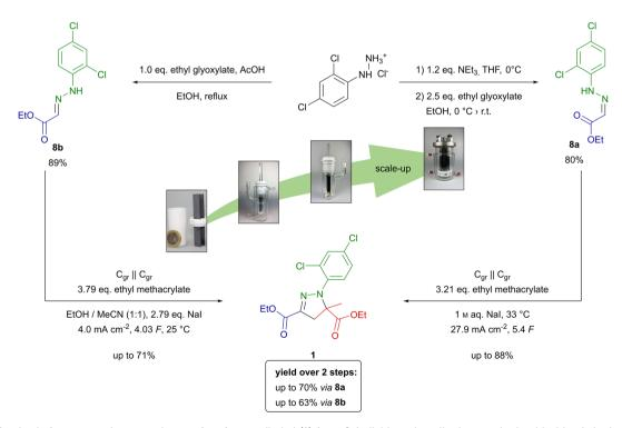
Scheme 2 Synthesis from screening to scale-up of mefenpyr-diethyl (1) from 2,4-dichlorophenylhydrazone hydrochloride via hydrazones 8a and
