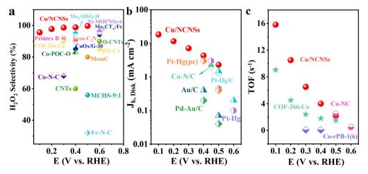
Fig. 3  $H_2O_2$  selectivity (a),  $J_k$  (b) and TOF (c) of Cu/NCNSs and other electrocatalysts reported in recent studies in alkaline media. Data adapted from: Au/C and Pd-Au/C ref. 52, Pt-Hg, Pt-Hg (pc) and Pt-Hg/C ref. 20, Co-N/C (heat-treated cobalt-porphyrin supported on vapor grown) ref. 53, Co-N/C ref. 13, COF-366-Co ref. 32, Co-rPB-1(6) ref. 50 and ref. in Table S3 (see ESI†) for the comparison of  $H_2O_2$  selectivity in alkaline media.
