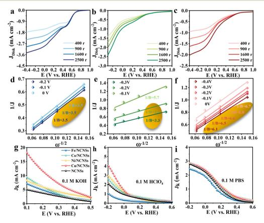
Fig. 4 Disk polarization curves of the Cu/NCNSs recorded in  $O_2$ -saturated 0.1 M KOH (a), 0.1 M HClO<sub>4</sub> solution (b) and 0.1 M PBS (c) at rotation rates between 400–2500 rpm, the corresponding K-L plots at different potentials in  $O_2$ -saturated 0.1 M KOH (d), 0.1 M HClO<sub>4</sub> (e) and 0.1 M PBS (f), and  $J_k$  values of the catalysts at 1600 rpm in 0.1 M KOH (g), 0.1 M HClO<sub>4</sub> (h) and 0.1 M PBS (i).
