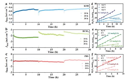
Fig. 6 Potentiostatic stability tests in 0.1 M KOH (a), 0.1 M HClO<sub>4</sub> (b) and 0.1 M PBS (c), H<sub>2</sub>O<sub>2</sub> yield rates of Cu/NCNSs obtained from different potentials in 0.1 M KOH (d), HClO<sub>4</sub> (e) and PBS (f).
