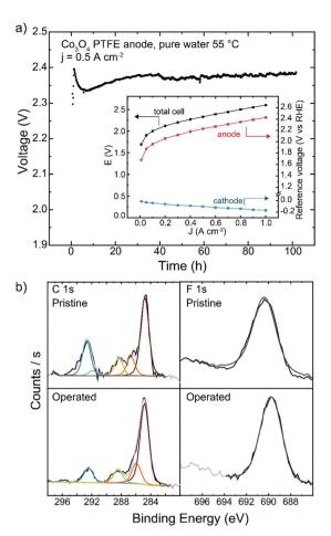
Fig. 10 Long-term operation of a PTFE-containing anode. (a) HEM electrolyzer operation with a Co<sub>3</sub>O<sub>4</sub>/20% PTFE-coated stainless-steel anode PTE, TP-85 membrane, and Pt-black/10% TP-85 cathode for 100 h at 55 °C. Inset shows cathode and anode contributions to total cell voltage. (b) XPS of the anode catalyst layer before and after 100 h operation.
