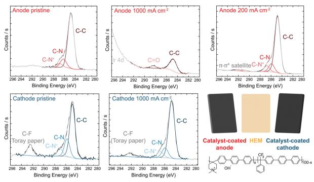
Fig. 4 XPS analysis of IrO<sub>x</sub>/20% TP-85 anode and Pt-black/10% TP-85 cathode. C 1s spectra of (a) anode and (b) cathode PTE. Inset shows the chemical structure of the TP-85 ionomer. Ionomer degradation is only observed on the anode PTE operating at high current.
