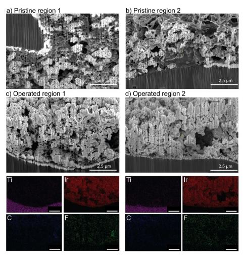
Fig. 9 Cross-sectional analysis of IrOx/mixed binder anode PTE. SEM images of different regions of the pristine catalyst layer (a) and (b) and SEM with EDX maps of two operated regions (c) and (d). Only PTFE binder is observed in the catalyst layer after operation.
