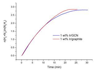
Fig. 1 Kinetic profiles of 1 wt% Ir/graphite (red) and 1 wt% Ir/GCN (blue) catalysts for hydrous hydrazine decomposition. All tests were performed at 323 K and 1400 rpm, using 300 μL of a hydrazine solution 3.3 M in 5 mL of NaOH 0.5 M and a  $N_2H_4\cdots H_2O$ : catalyst molar ratio of 1000:1. A sampling time of 0.3 s was employed to obtain continuous kinetic profiles.
