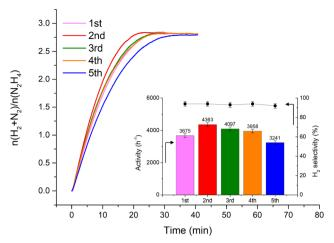
Fig. 3 Stability tests for 1 wt% Ir/GCN. The insets are the catalytic activity (left axis) and  $\rm H_2$  selectivity (right axis) trends along repeated cycles. All tests were performed at 323 K and 1400 rpm, using 300  $\rm \mu L$  of a 3.3 M hydrazine solution in 5 mL of 0.5 M NaOH and a  $\rm N_2H_4\cdots H_2O$ : catalyst molar ratio of 1000:1. A sampling time of 0.3 s was employed to obtain continuous kinetic profiles.
