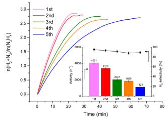
Fig. 2 Stability tests for 1 wt% Ir/graphite. The insets are the catalytic activity (left axis) and H2 selectivity (right axis) trends along repeated cycles. All tests were performed at 323 K and 1400 rpm, using 300 µL of a 3.3 M hydrazine solution in 5 mL of 0.5 M NaOH and a N<sub>2</sub>H<sub>4</sub>···H<sub>2</sub>O: catalyst molar ratio of 1000:1. A sampling time of 0.3 s was employed to obtain continuous kinetic profiles.
