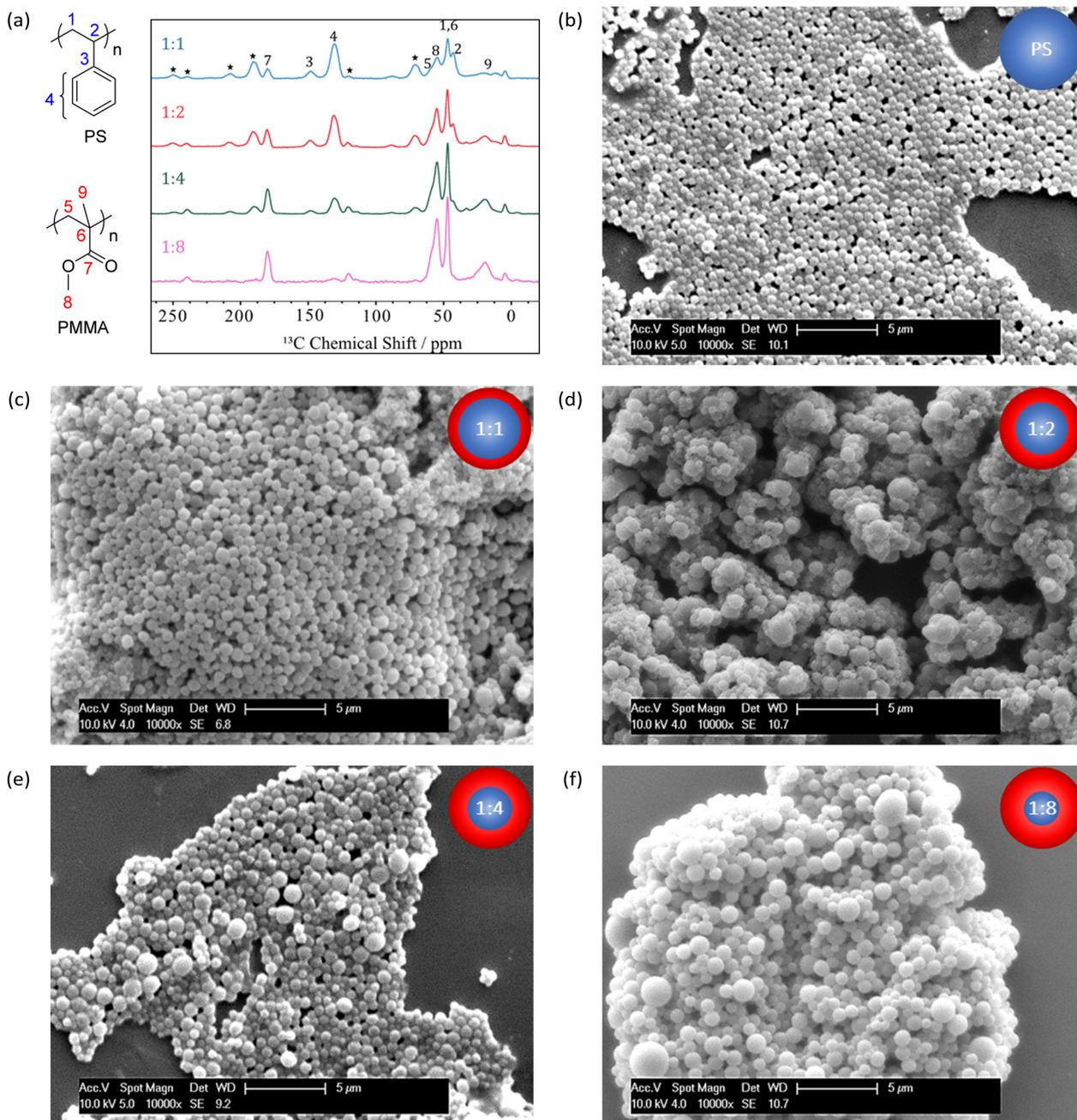
**Fig. 2** (a)  $^1\text{H}$ - $^{13}\text{C}$  CP-MAS spectra of PS-PMMA core-shell polymers with PS:PMMA ratios of 1:1, 1:2, 1:4 and 1:8 (note: spinning sidebands marked with \*, inset shows numbering of  $^{13}\text{C}$  assignments), and SEM micrographs of (b) PS particles (core), and PS-PMMA core-shell particles with targeted mass ratios of (c) 1:1, (d) 1:2, (e) 1:4 and (f) 1:8.
