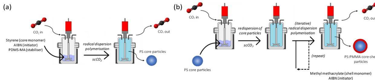
Fig. 1 Reaction schematic of (a) PS core and (b) PMMA shell syntheses in supercritical CO<sub>2</sub> in a high-pressure autoclave.
