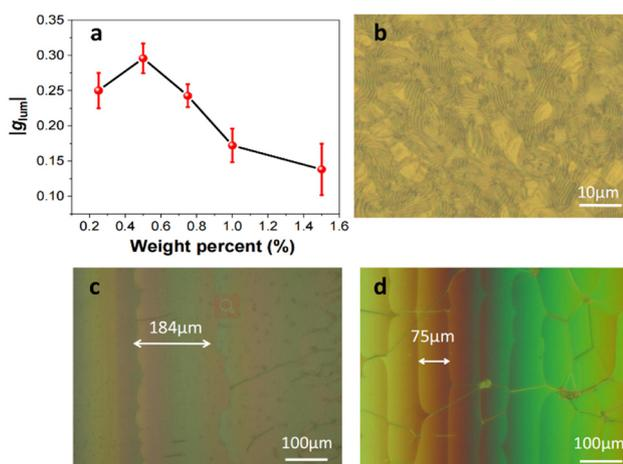
Fig. 2 (a) The tendency of CPL  $g_{lum}$  values with different mixing weight ratios of *R*-1-C,  $\lambda_{ex} = 360$  nm, all error bars show the mean  $\pm$  standard deviation,  $n = 5$  independent experiments. (b) POM image of *R*-1-C/E7, [*R*-1-C] = 0.5 wt%. POM images of N\*-LC including 0.5 wt% (c) *R*-1-O and (d) *R*-1-C in wedge-shaped cells at room temperature.
