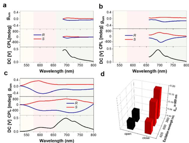
Fig. 4 (a–c) CPL spectra of *R(S)*-1-C-NR-Cy5 cholesteric texture ( $\lambda_{\text{ex}} = 625$  nm,  $\lambda_{\text{ex}} = 550$  nm,  $\lambda_{\text{ex}} = 360$  nm, respectively). (d) 3D Column diagrams of CPL  $g_{\text{lum}}$  values obtained by irradiation of donor *R*-1 or acceptor dyes when CET was turned “on” and “off”, respectively.
