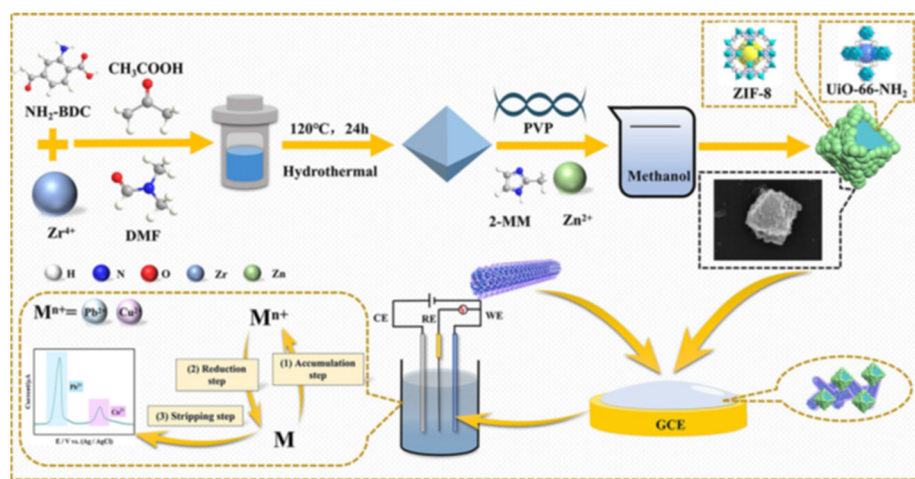
Fig. 5 The synthesis route of NU66@Z8 and the construction of the working electrode 150 (this figure was published in R. Tan, P. Jiang, C. Pan, J. Pan, N. Gao, Z. Cai, F. Wu, G. Chang, A. Xie, Y. He, Core-shell architected NH 2 -UIO-66@ZIF-8/multi-walled carbon nanotubes nanocomposite-based sensitive electrochemical sensor towards simultaneous determination of Pb 2+ and Cu 2+ , Microchim. Acta , 190 , 30, Copyright Springer (2023)).
