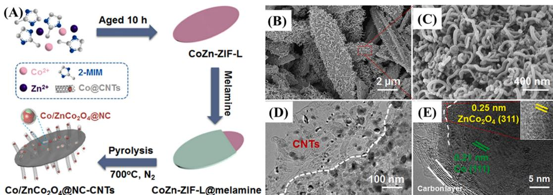
Fig. 20 (A) Schematic synthesis process of the  $\text{Co/ZnCo}_2\text{O}_4@NC\text{-CNT}$  electrocatalyst. (B and C) SEM images, (D) TEM image, and (E) HRTEM image of the as-prepared  $\text{Co/ZnCo}_2\text{O}_4@NC\text{-CNTs}$ . Reproduced with permission.<sup>255</sup> Copyright © 2020 Elsevier Ltd. All rights reserved.
