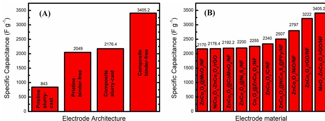
Fig. 13 (A) Best specific capacitance for each ZnCo<sub>2</sub>O<sub>4</sub>-based electrode type: pristine slurry-cast; pristine binder-free; composite slurry-cast and composite binder-free (ref. 11, 26, 58 and 62, respectively). (B) Top 10 specific capacitances delivered by ZnCo<sub>2</sub>O<sub>4</sub>-based electrodes (ref. 62, 43, 38, 90, 84, 67, 75, 79, 58 and 89, respectively).
