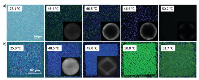
Fig. 7 Chirality Induction by the addition of chiral dopant S811 in a mixture of 13.0 wt% RM257 and BP: (a) hybrid confinement; scale bar: 100 µm; (b) directed self-assembly; scale bar: 200 µm.
