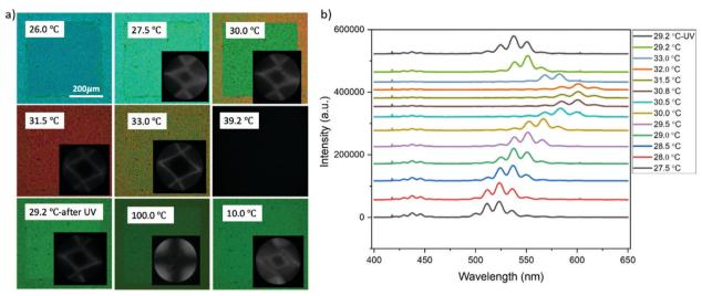
Fig. 6 Polymer stabilization of BPLC on the chemically patterned substrate: (a) POM images of the sample's (RM82/TMPTA/Irg651: 9.3/2.7/0.38 wt%) thermal cycle before polymerization, and BPLC thermal stability after polymerization. Scale bar: 200 µm. (b) The correlation between the wavelength and intensity of RM82/TMPTA/Irg651: 9.3/2.7/0.38 wt% as a function of temperature.
