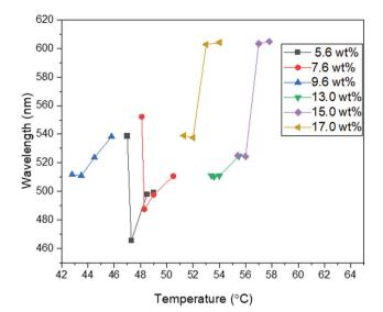
Fig. 5 The wavelength of intensity peaks vs. temperature for different concentrations of RM82 in directed self-assembly
