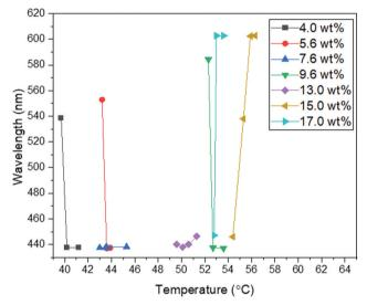
Fig. 3 The relative wavelength vs. temperature for RM82 weight fractions in hybrid cell confinement.
