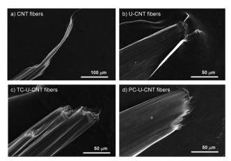
Fig. 4 Fractographic SEM images of (a) CNT, (b) U-CNT, (c) TC-U-CNT, and (d) PC-U-CNT fibers.
