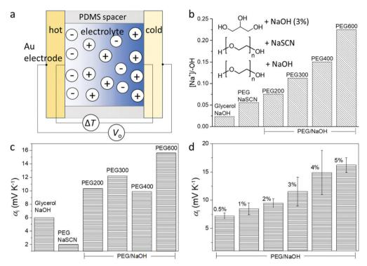
Fig. 2 Illustration of the ionic thermoelectric device and involved materials. (a) The structure of the ionic thermoelectric device. (b) The composition of the studied electrolytes with 3 wt% of salts. (c) The Seebeck coefficient of electrolytes containing different salts (3 wt%) and solvents. (d) The Seebeck coefficient of NaOH/PEG(400) electrolytes of different NaOH concentration.
