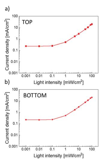
Fig. 4 Linearity (current density vs. light power) of the semitransparent (ITO top contact) MA<sub>0.3</sub>FA<sub>0.7</sub>Pb<sub>0.5</sub>Sn<sub>0.5</sub>I<sub>3</sub> perovskite photodetector illuminated from the (a) top and (b) bottom.
