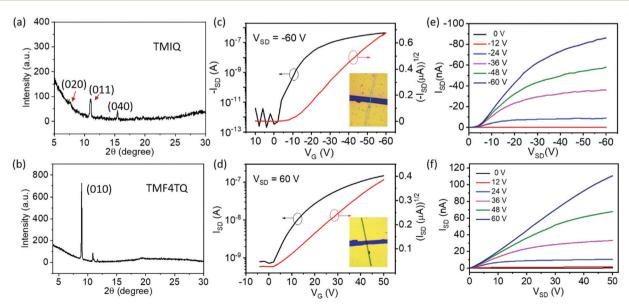
Fig. 4 (a and b) XRD patterns of self-assembled microcrystals for (a) TMIQ and (b) TMF4TQ on OTS-modified SiO<sub>2</sub>/Si substrates. (c and d) Representative transfer and (e and f) output characteristics of OFET devices based on (c and e) TMIQ and (d and f) TMF4TQ micro-ribbons (inset: the corresponding device)
