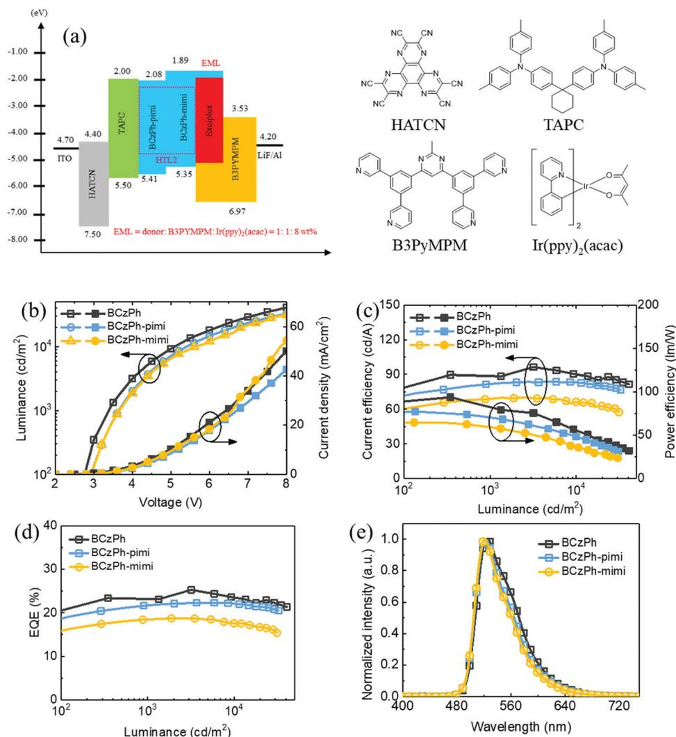
**Fig. 4** (a) Energy level diagrams and molecular structures of devices, (b) current density–voltage–luminance ( $J$ – $V$ – $L$ ) of devices with an exciplex as the host, (c) Current and power efficiency of devices with an exciplex as the host, (d) External quantum efficiency (EQE) versus luminance of devices with an exciplex as the host and (e) EL spectra of devices with an exciplex as the host, for PhOLEDs.
