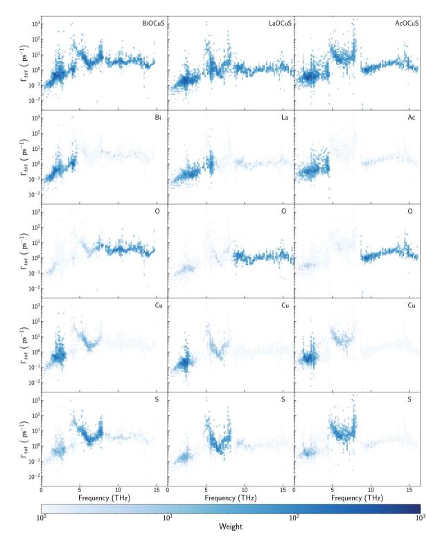
Fig. 4 Scattering rates—frequency heat maps for BiOCuSe (top left), LaOCuS (top mid), and AcOCuS (top right) at 300 K. Heat map color represents the density of vibrational modes with similar scattering rates and frequencies. Projections on each element have been depicted below the total contributions.
