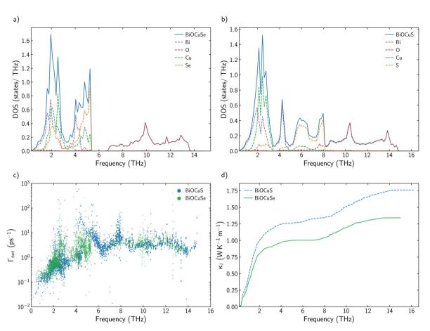
Fig. 2 (a and b) Total and projected phonon density of states, DOS, of BiOCuSe and BiOCuS. (c) Total scattering rates,  $\Gamma_{\text{tot}}$  for BiOCuSe (green) and BiOCuS (blue) at 300 K. (d) Cumulative  $\kappa_{\text{I}}$  for BiOCuSe (green solid line) and BiOCuS (blue dashed line) at 300 K.
