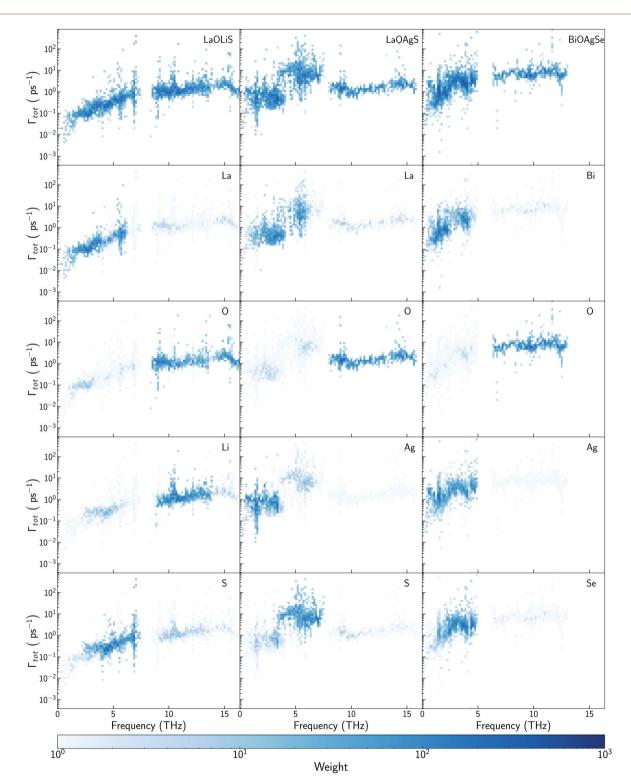
Fig. 6 Scattering rates—frequency heat maps for LaOLiS (top left), LaOAgS (top mid), and BiOAgSe (top right). Heat map color represents the density of vibrational modes with similar scattering rates and frequencies. Projections on each element have been depicted below the total contributions.
