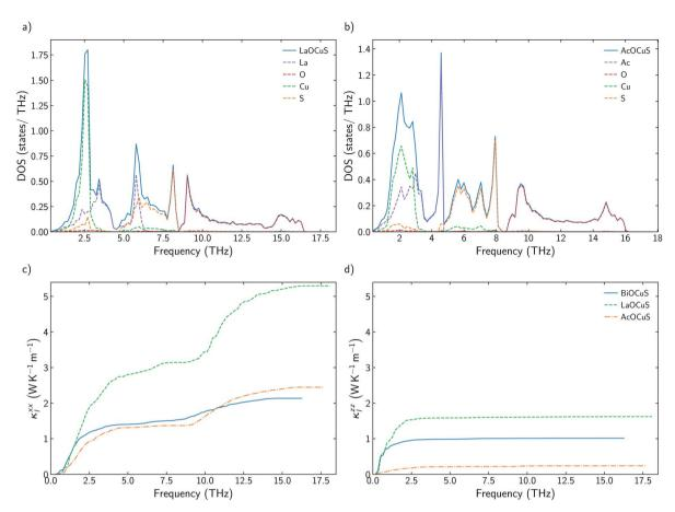
Fig. 3 (a and b) Total and projected phonon density of states, DOS, of LaOCuS and AcOCuS. (c and d) Cumulative  $\kappa_1^{xx}$  and  $\kappa_2^{zz}$  for BiOCuSe, LaOCuS, and AcOCuS at 300 K.
