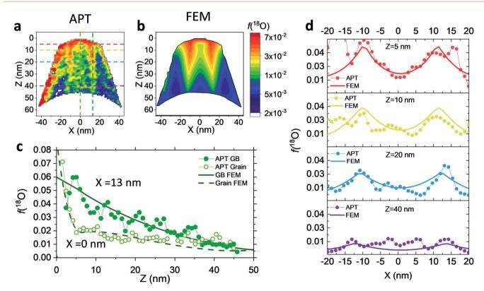
Fig. 2 D vertical cross section of the <sup>18</sup>O fraction measured by APT (a) and obtained by FEM simulations (b). (c) 1D out-of-plane profiles of the isotope fraction obtained along a GB and along the grain bulk of the LSM tip, as measured by IE-APT and calculated in the FEM simulation. (d) 1D horizontal <sup>18</sup>O fraction measured at different distances from the sample's surface. The vertical and horizontal 1D profiles shown in (c) and (d) are depicted in a as dashed lines.
